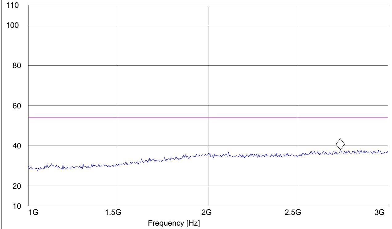
**3-18GHz****Note: Peak Reading vs. Average limit****Note: This plot shows worse case emission for low, mid, and high channel.**
