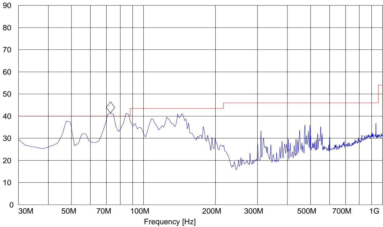
**30MHz – 1GHz****Antenna: horizontal.****Note: This plot shows worse case emission for low, mid, and high channel.**
