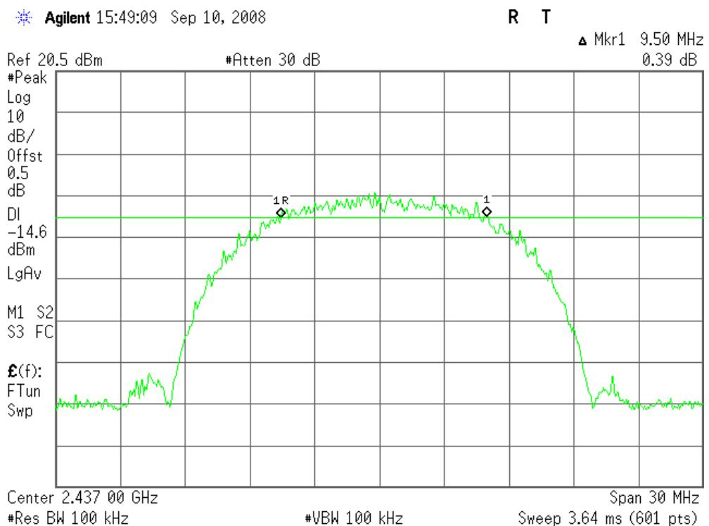
**6dB Bandwidth (CH High)**
