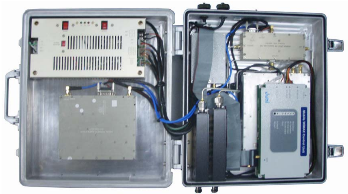
[Figure 6] Mobile WiMAX Repeater' s Interior
