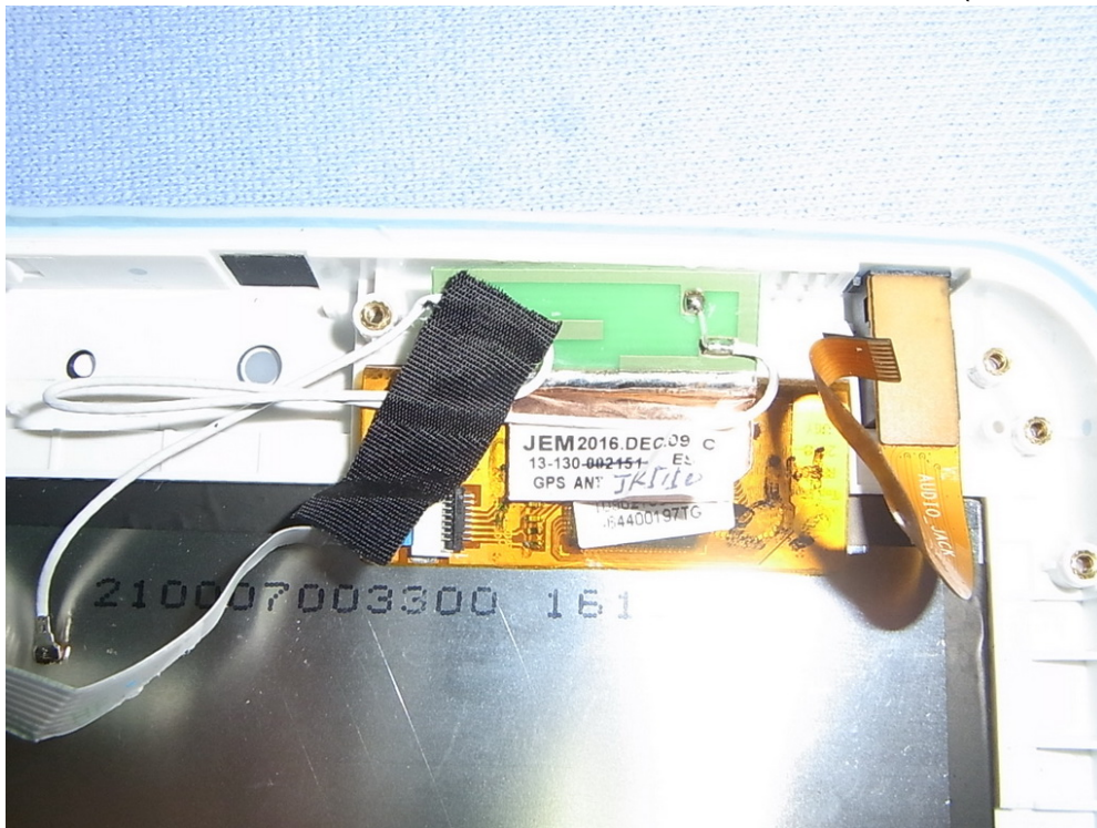
Figure 46 7" Multi Function Pad, Internal View (GPS Antenna)
