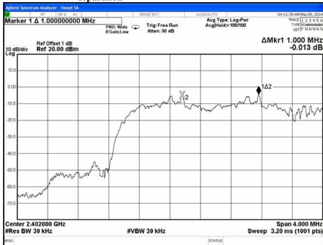
**Test Mode: 8-DPSK, 2441MHz adjacent channel of right carrier frequency separation**
