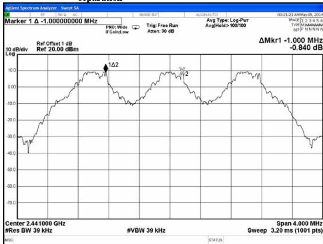
**Test Mode: GFSK, 2441MHz adjacent channel of left carrier frequency separation**
