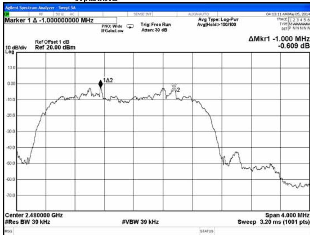
**Test Mode: GFSK, 2402MHz adjacent channel of carrier frequency separation**
