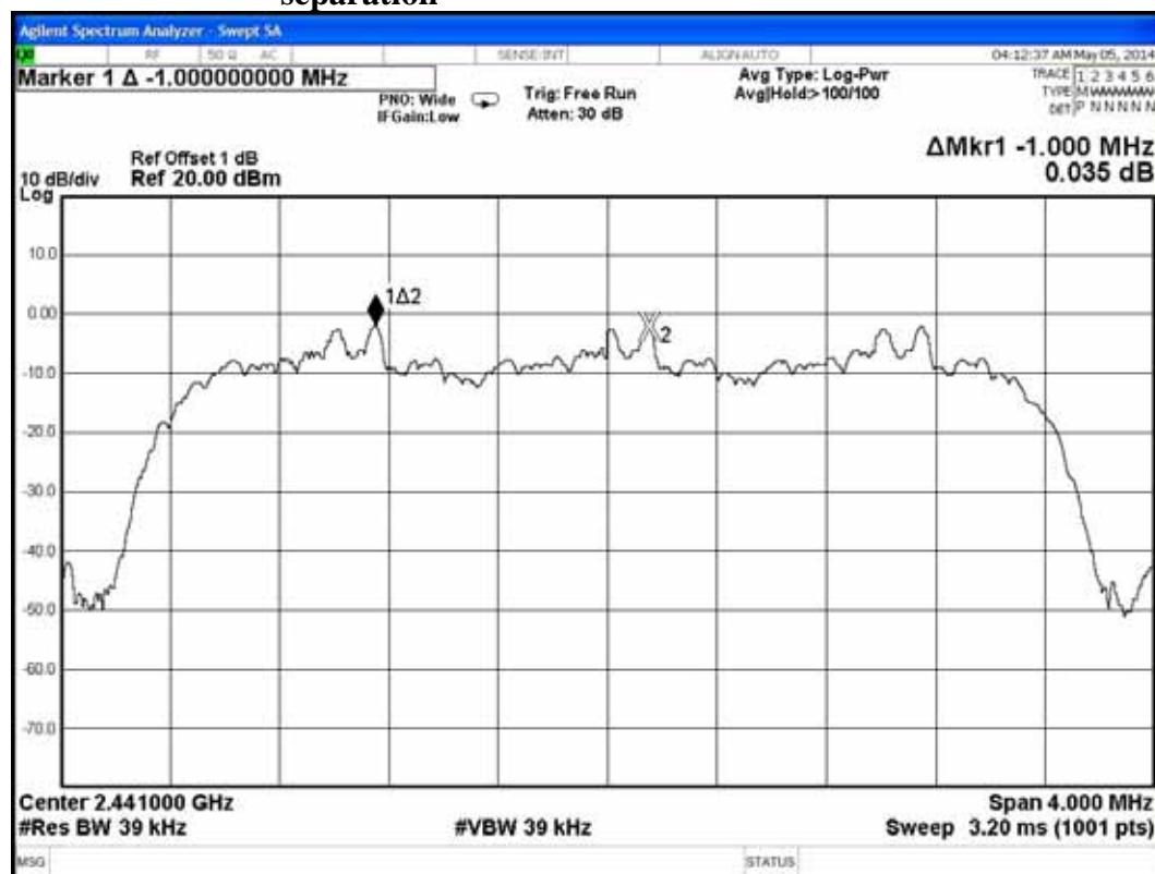
**Test Mode: 8-DPSK, 2441MHz adjacent channel of left carrier frequency separation**
