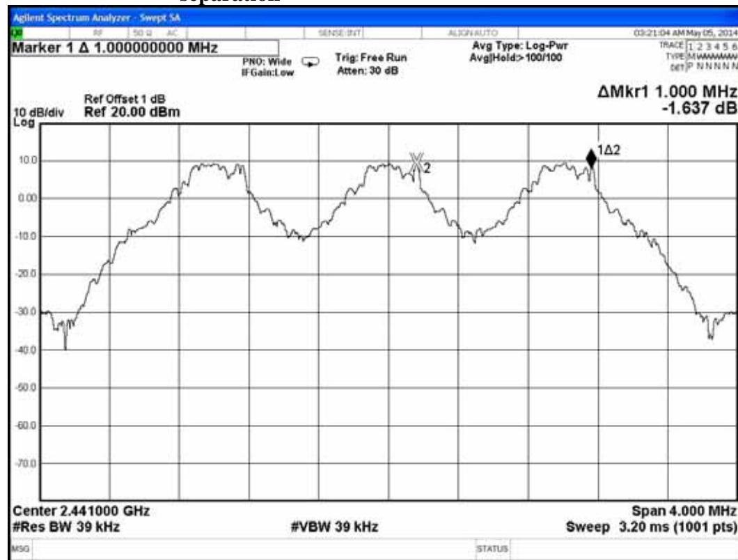
**Test Mode: GFSK, 2480MHz adjacent channel of carrier frequency separation**
