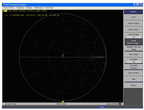
Calibrated return loss: -20.9 dB; Measured return loss: -20.7dB (within 20%)
