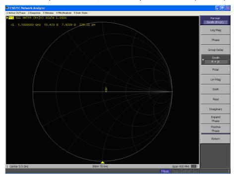
Calibrated return loss: -25.3 dB; Measured return loss: -23.47dB (within 20%)
