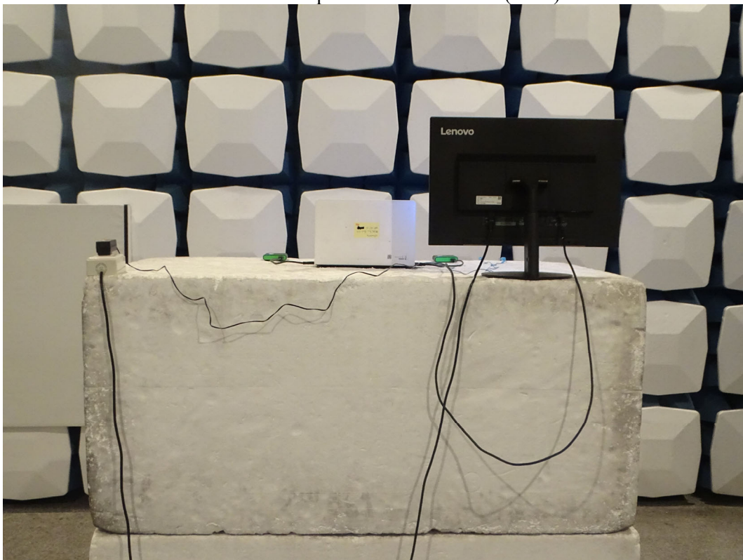
Back View of Spurious Emission Test (Horn)
