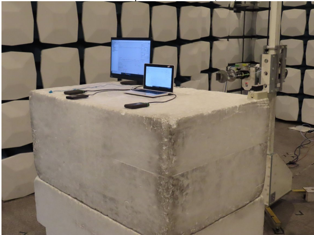
Front View of Spurious Emission Test (Horn)
