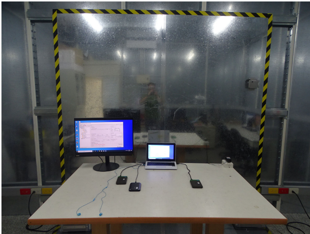
Front View of Conducted Test
