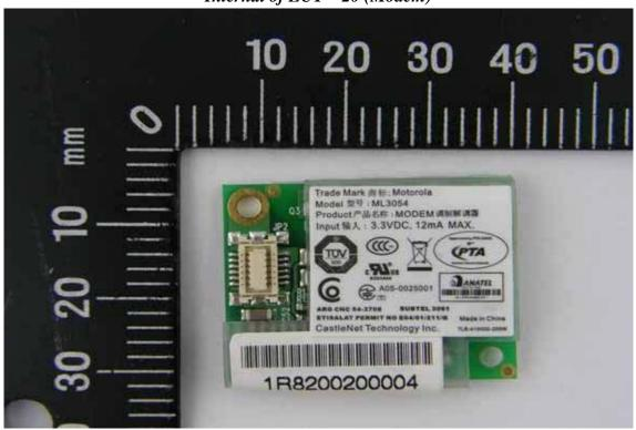
Internal of EUT – 21 (Modem)
