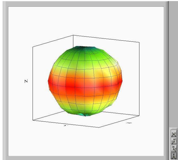
Max Antenna 3D Radiation Pattern 5150-5250 MHz
