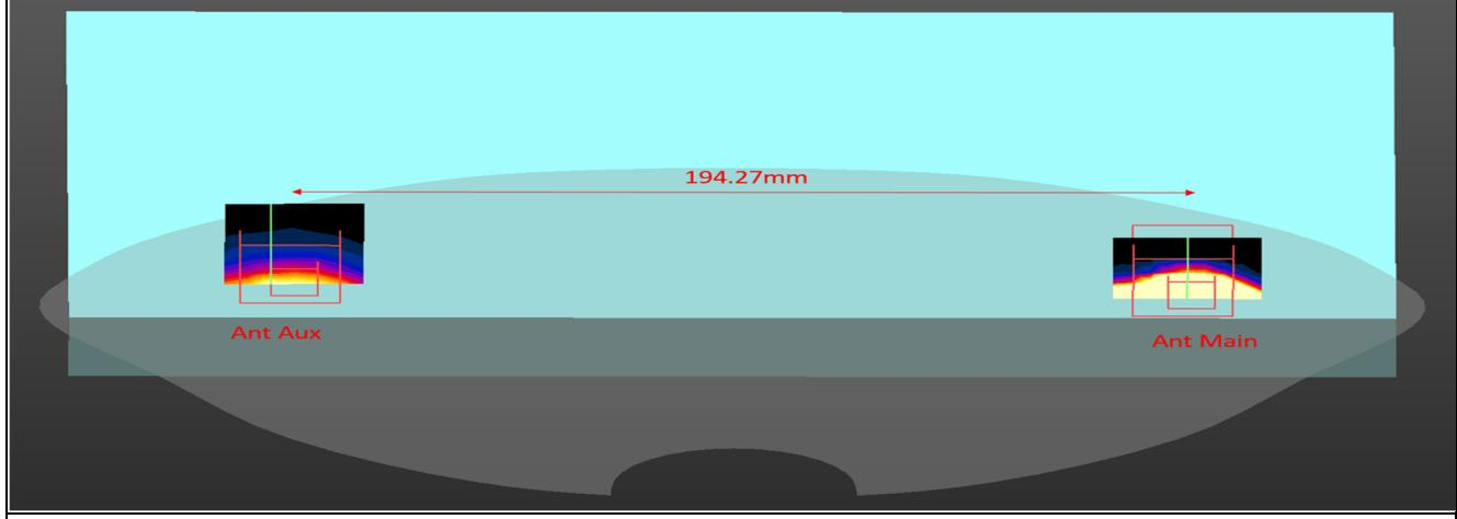
The ratio of value is less than 0.04, thus simultaneous SAR testing is not needed.
