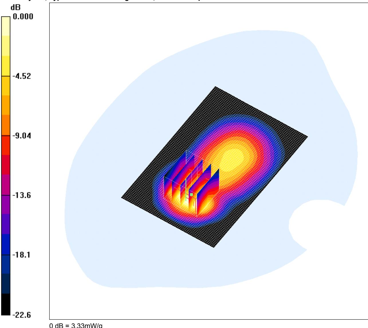
Communication System: PCS 1900; Frequency: 1879.8 MHz; Duty Cycle: 1:8.3
