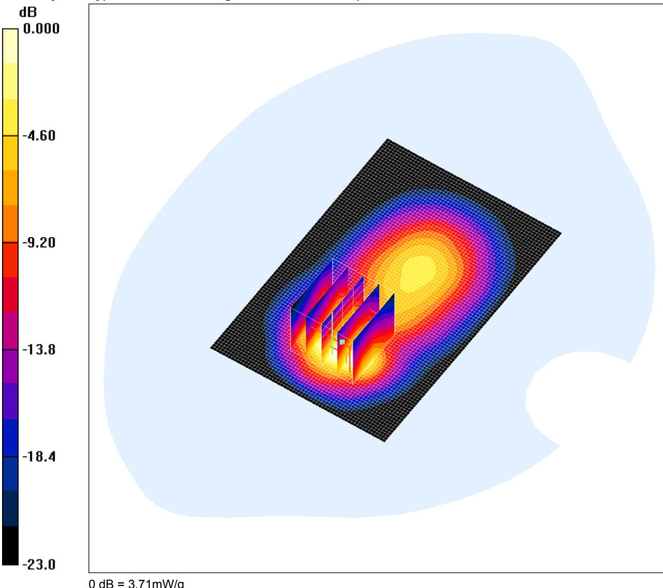
Communication System: PCS 1900; Frequency: 1909.8 MHz; Duty Cycle: 1:8.3
