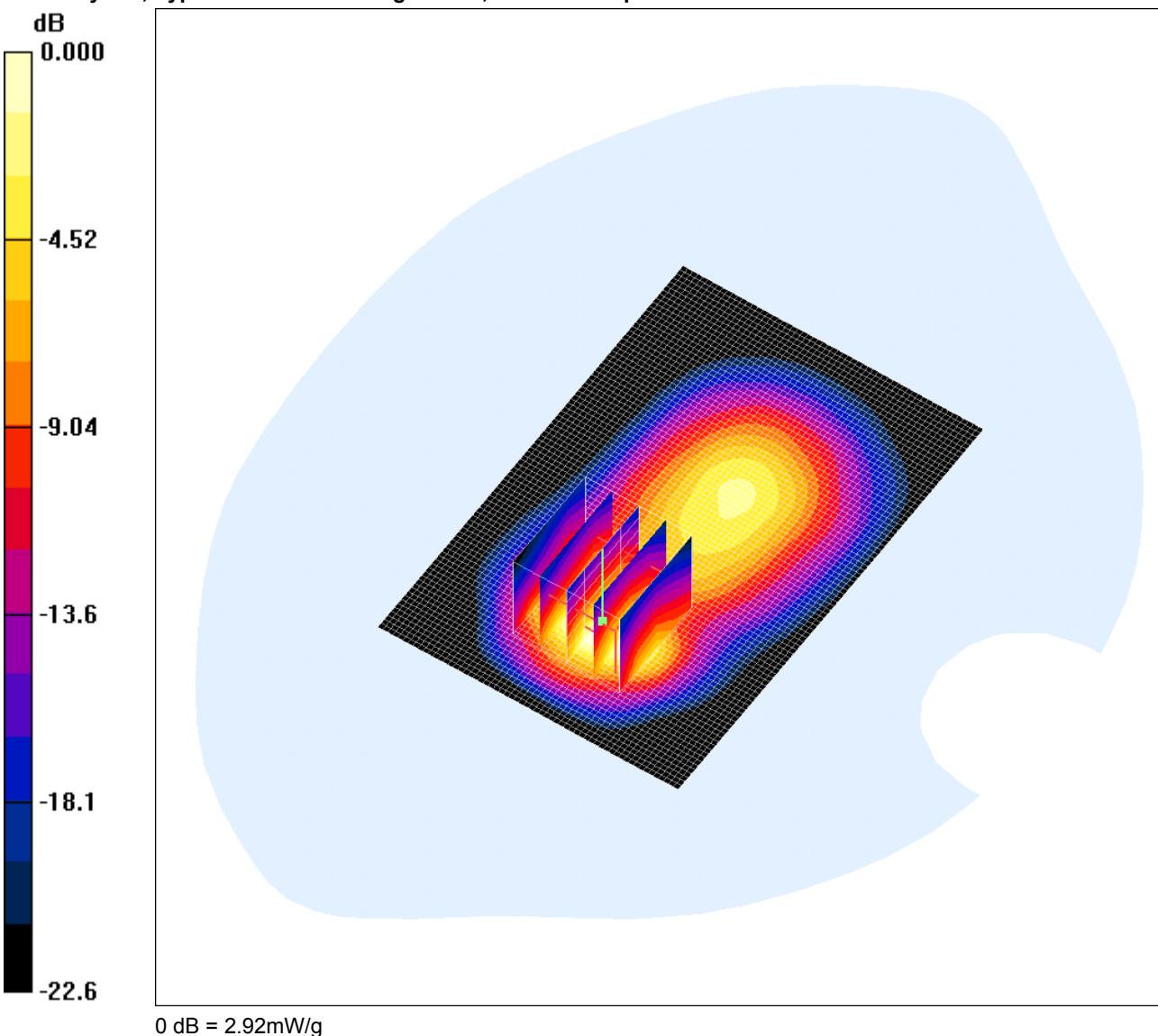
Communication System: PCS 1900; Frequency: 1850.2 MHz; Duty Cycle: 1:8.3
