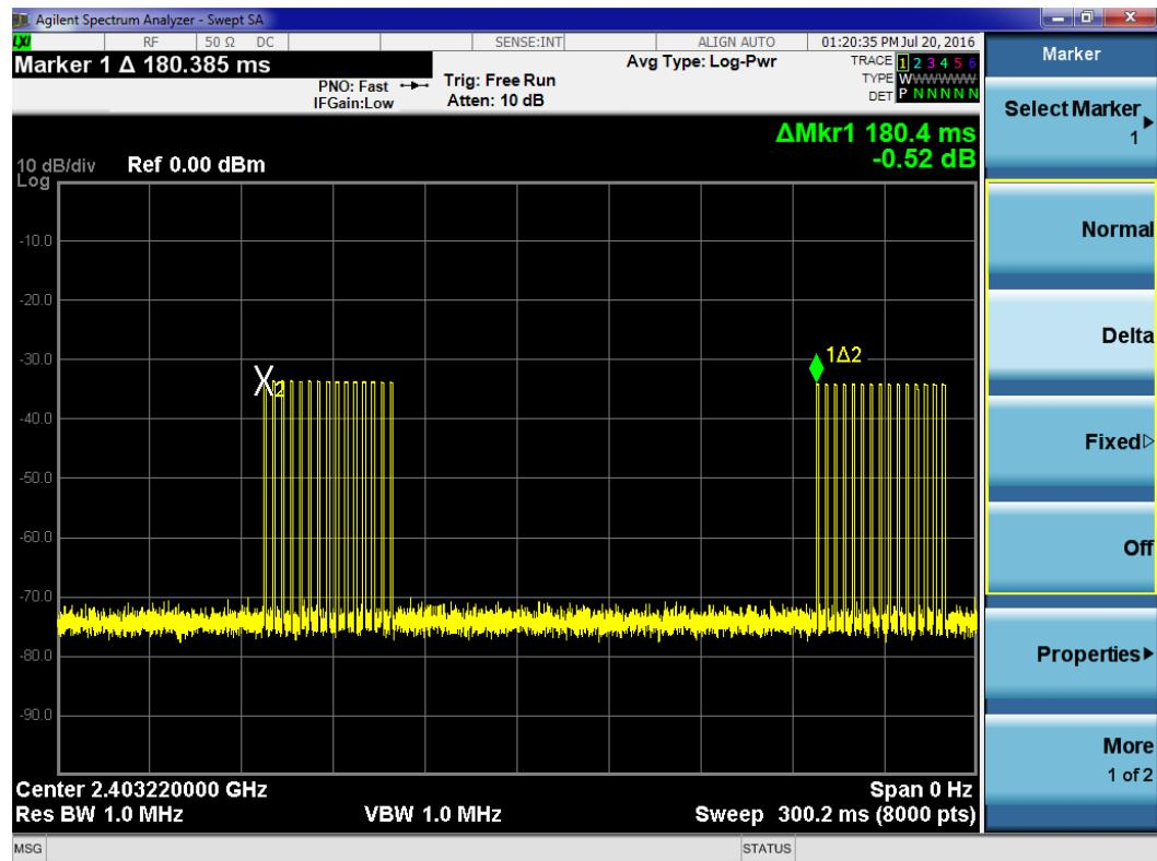
total 15 burst in 1 cycle, 180.4ms for 1cycle
