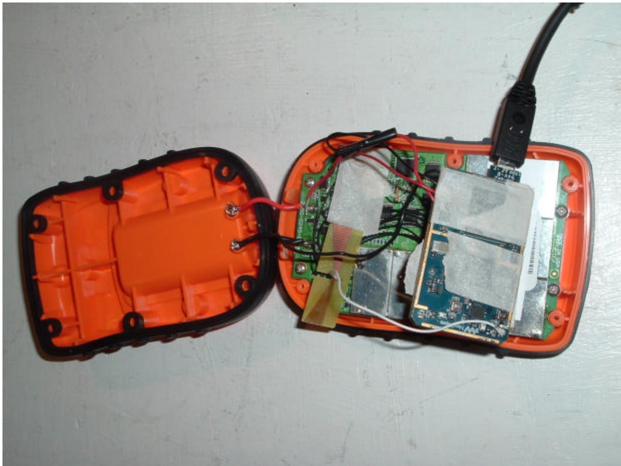
**Note: WiMax module and control circuitry insulated using thin, non-conductive tape to prevent shorting of circuitry during testing.**
