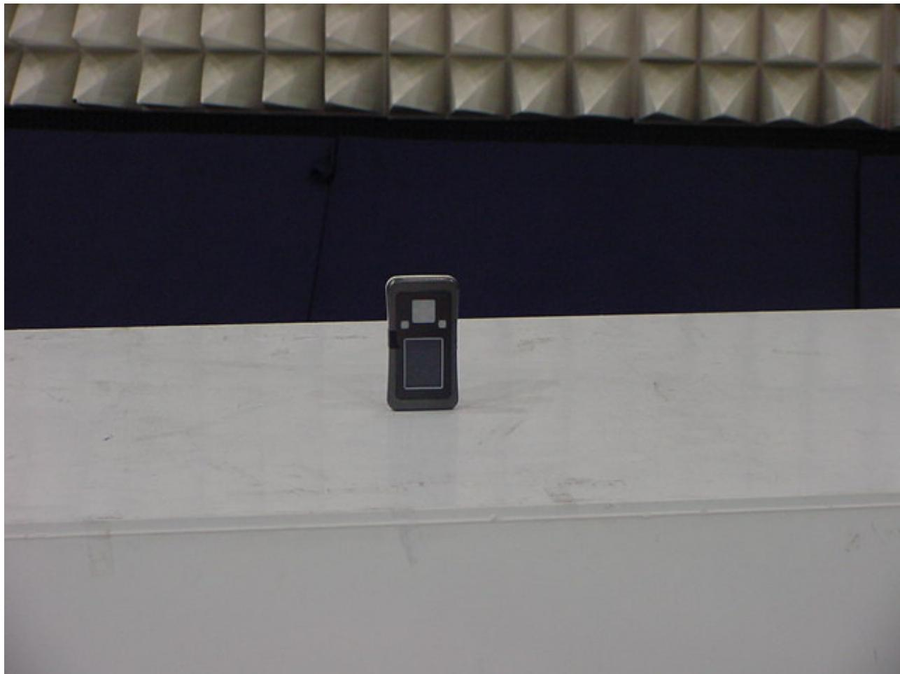
Radiated emission test
