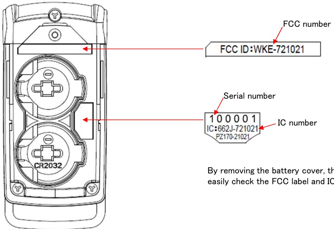
By removing the battery cover, the user can easily check the FCC label and IC label.
