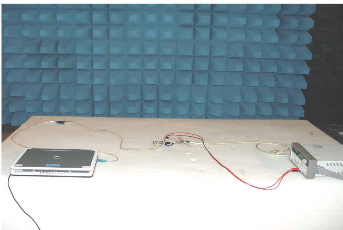
**POWERLINE CONDUCTED EMISSIONS SETUP PHOTOS**
