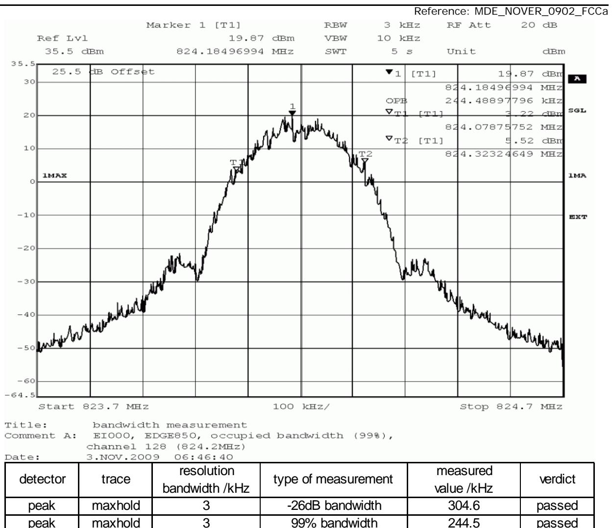
Test: 22.5; Frequency Band = 850, Mode = EDGE, Channel = 190, Frequency = 836.6MHz
