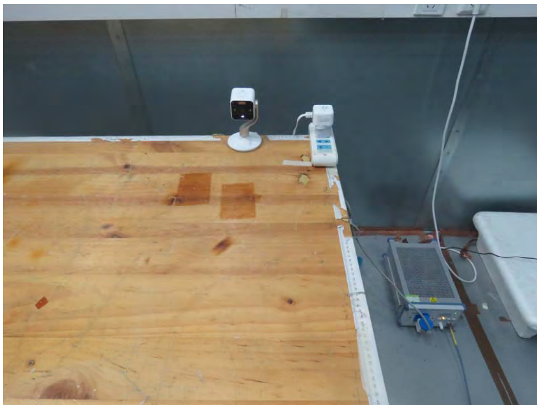
Picture 3 Conducted Emission Test Setup
