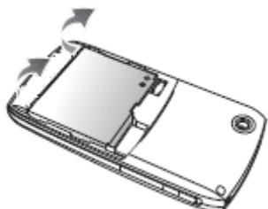
1. Slide the battery cover and remove the battery to the arrow direction as shown in the figure
