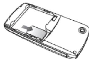
2. Face the gold color contact point of SIM card towards the cellular phone and push in the SIM card into the slot at the exact position.
