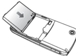
3. Align the gold color part of the battery to the groove marked with the gold color at the rear side of the phone as shown in the figure.
