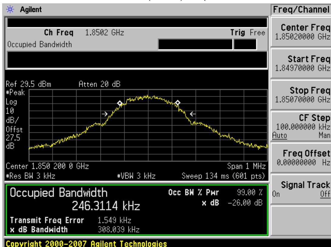
■ GSM1900 MODE (661 CH.) Occupied Bandwidth
