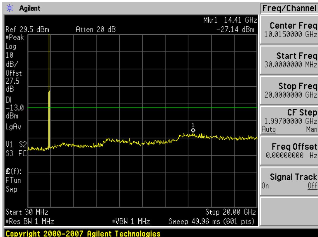
■ GSM1900 MODE (810 CH.) Conducted Spurious Emissions
