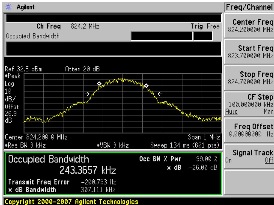
■ GSM850 MODE (190 CH.) Occupied Bandwidth
