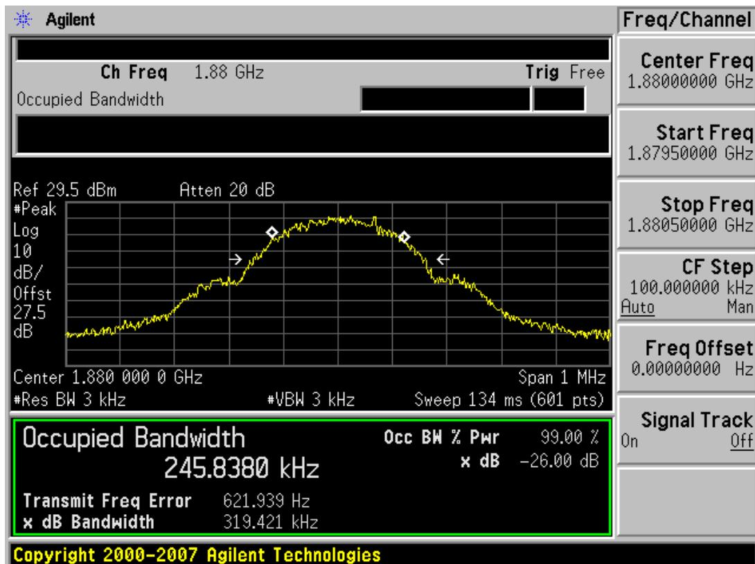
■ GSM1900 MODE (810 CH.) Occupied Bandwidth
