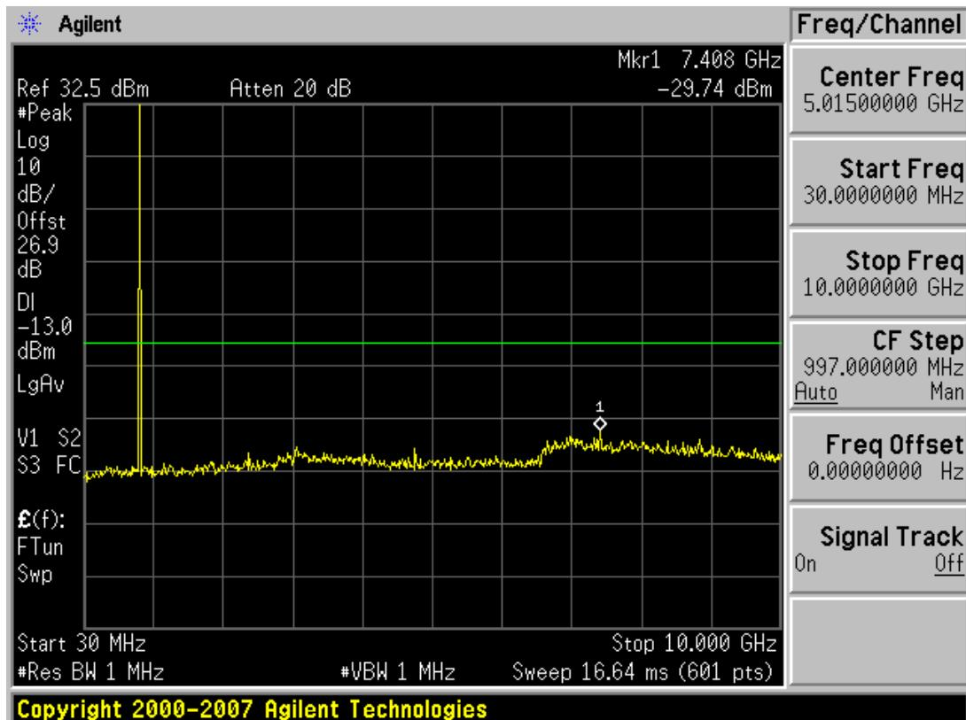
■ GSM850 MODE (190 CH.) Conducted Spurious Emissions
