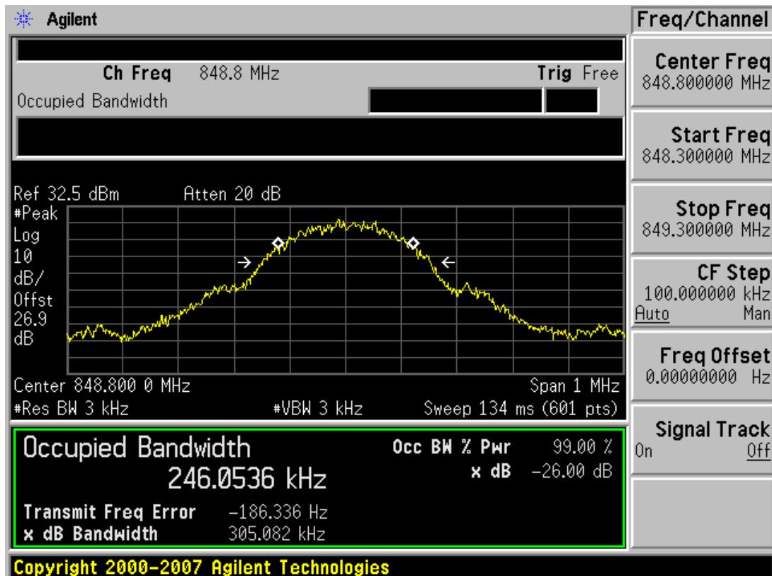
■ GSM1900 MODE (512 CH.) Occupied Bandwidth
