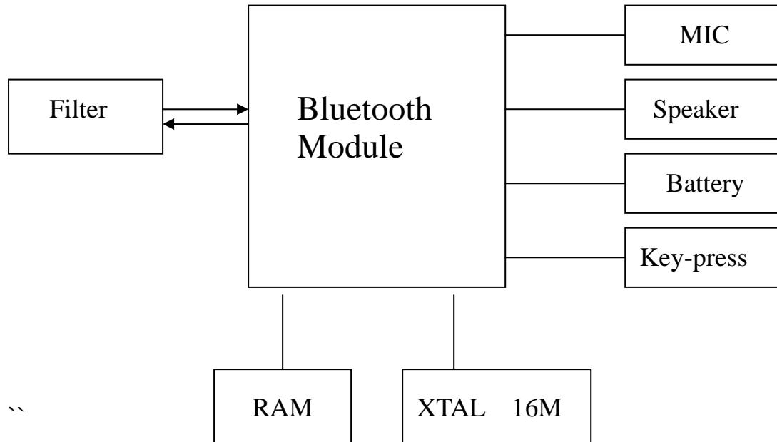
2. The Mobile Wireless Headset uses a short-range wireless communication Technology. The design applied is in in ternational identification ISM (Industrial Scientific and Medical )frequency bandwidth environment that is 2.4GHz—2.48GHz bandwidth.
