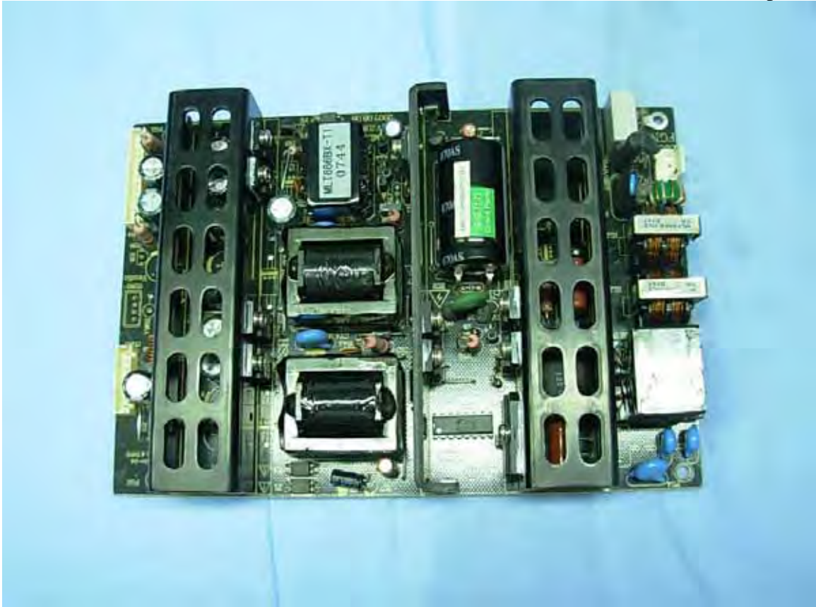
Figure 14 Power Board (Component Side)
