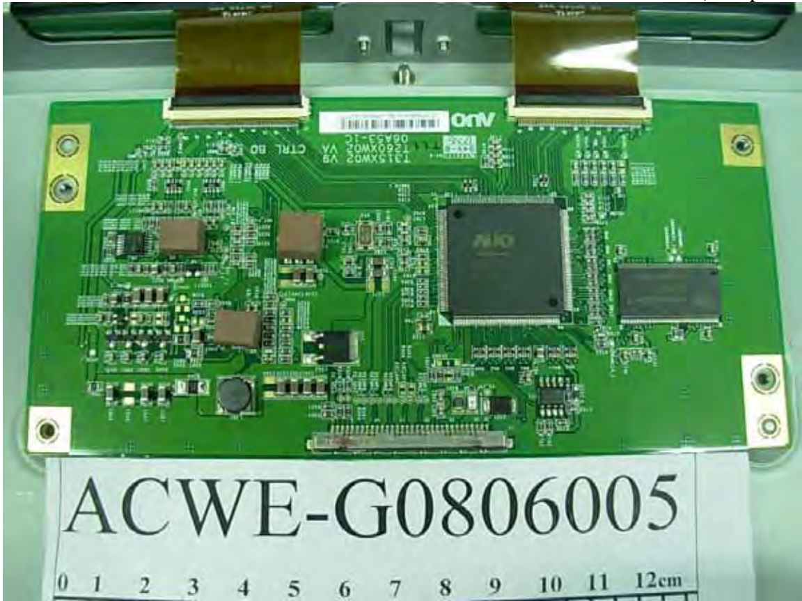
Figure 22 Control Board (Component Side)
