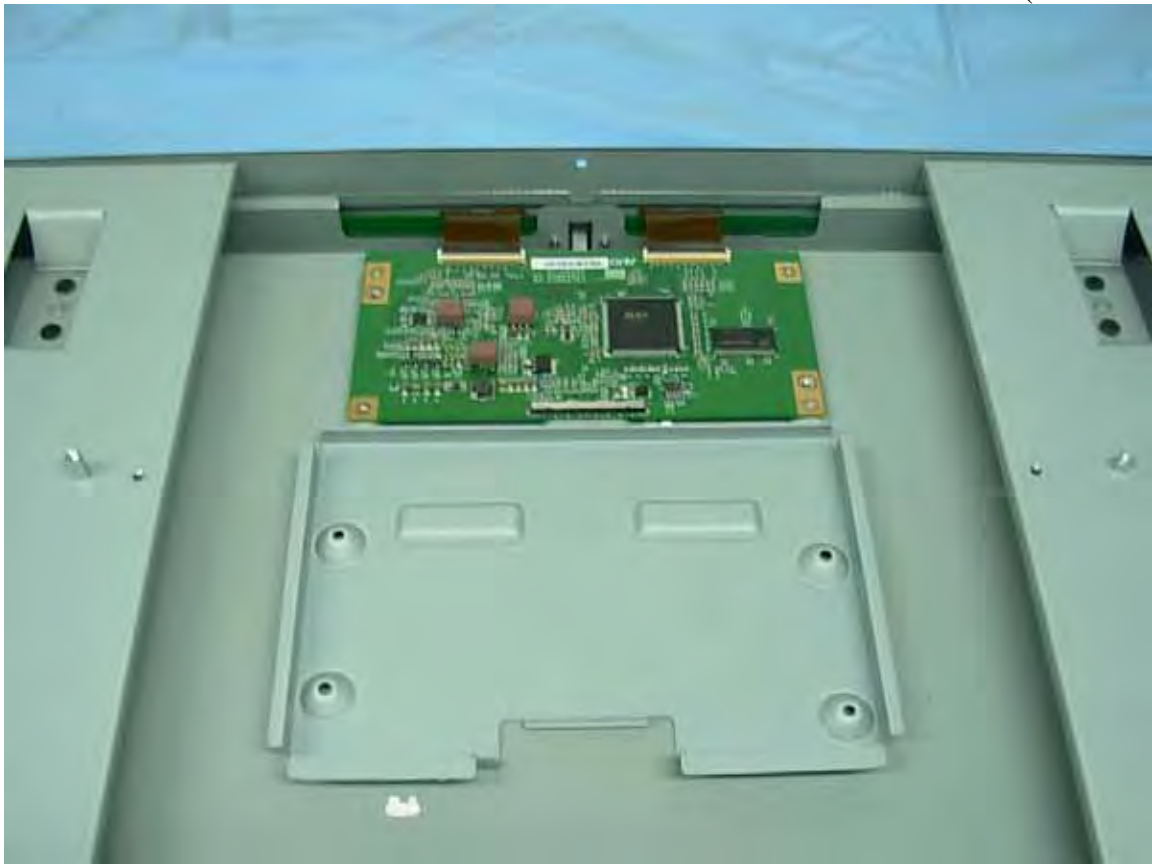
Figure 22 Control Board (Component Side)
