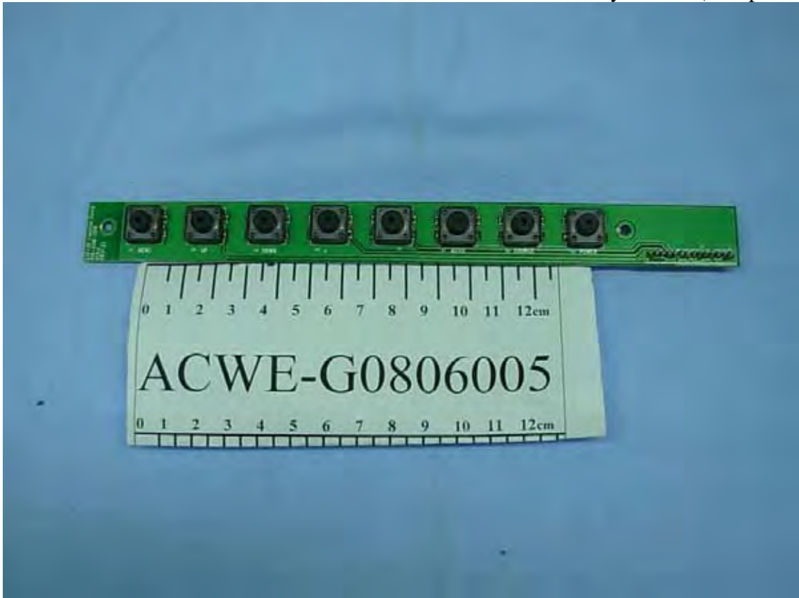
Figure 4 Key Board (Component Side)
