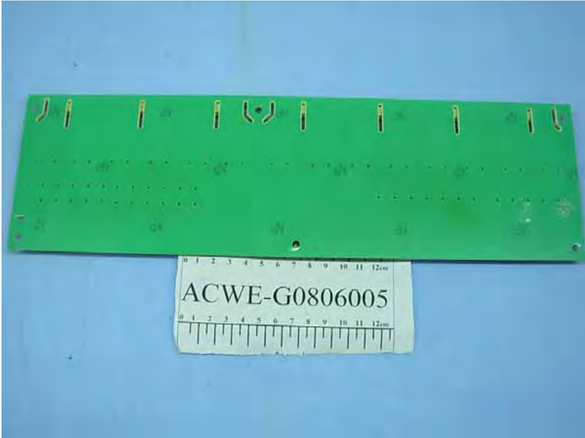
Figure26 Inverter Board (Solder Side)
