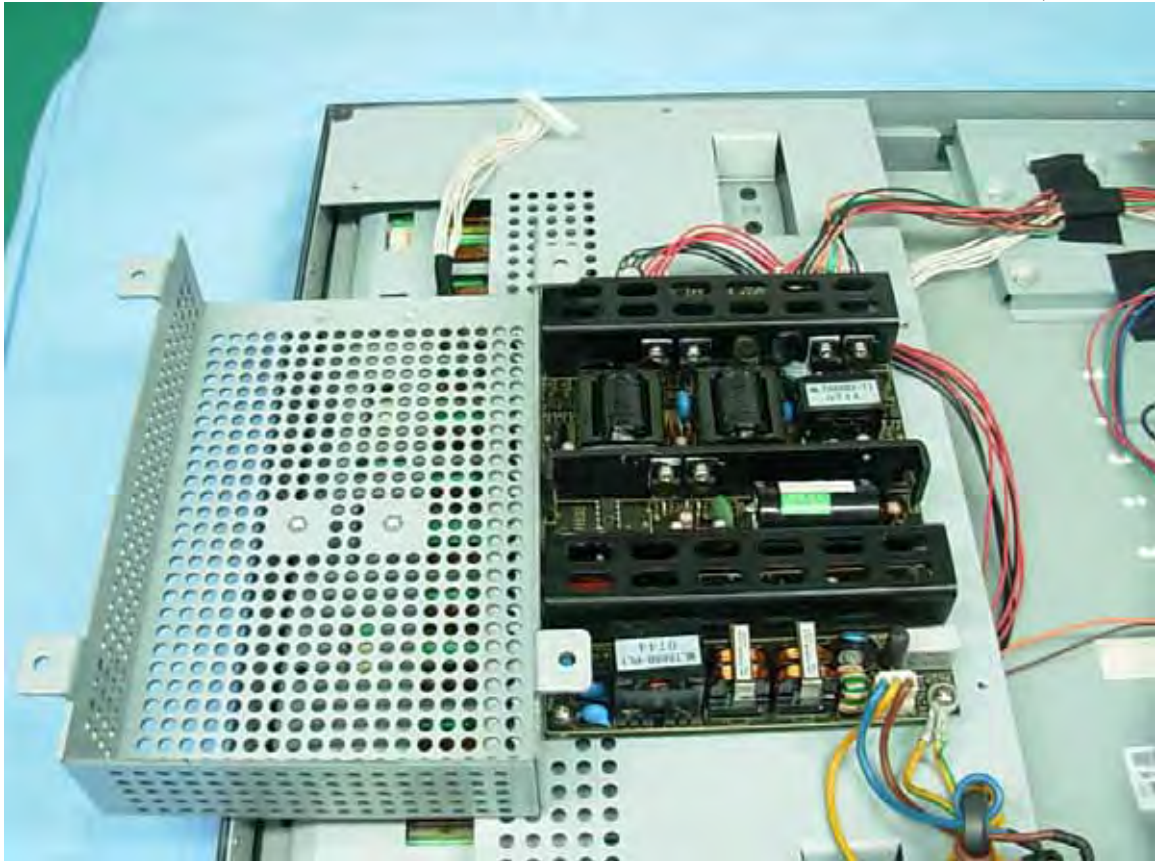
Figure 14 Power Board (Component Side)
