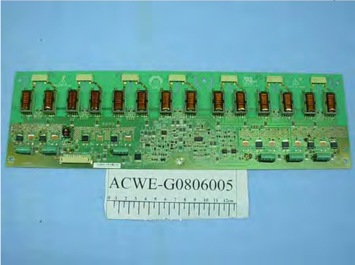
Figure26 Inverter Board (Solder Side)
