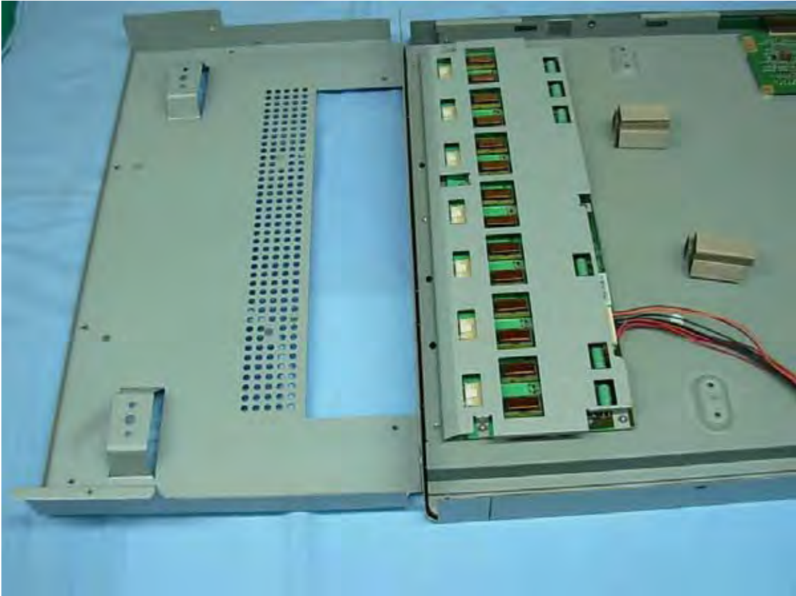
Figure 24 Inverter Board (Cover Remove)
