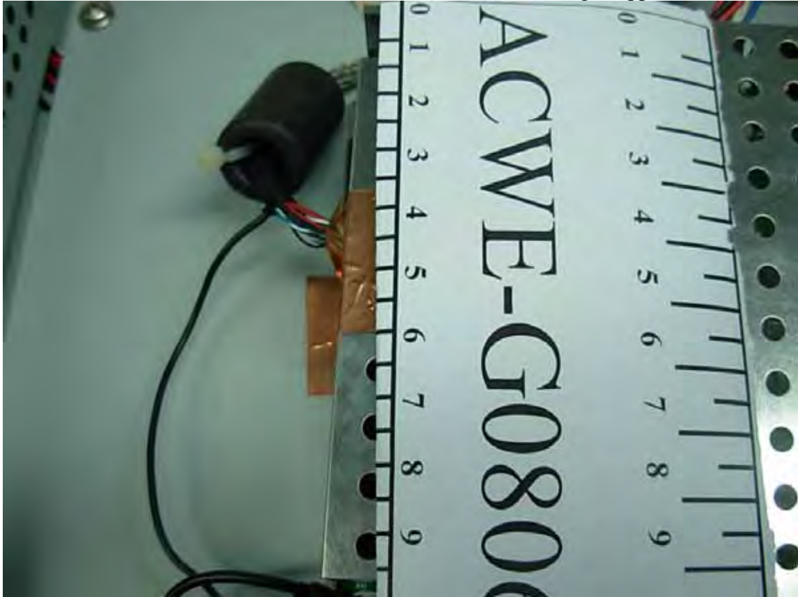
Figure 34 Conducting Copper Foil & Ferrite Core
