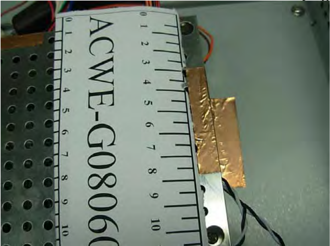
Figure 34 Conducting Copper Foil & Ferrite Core
