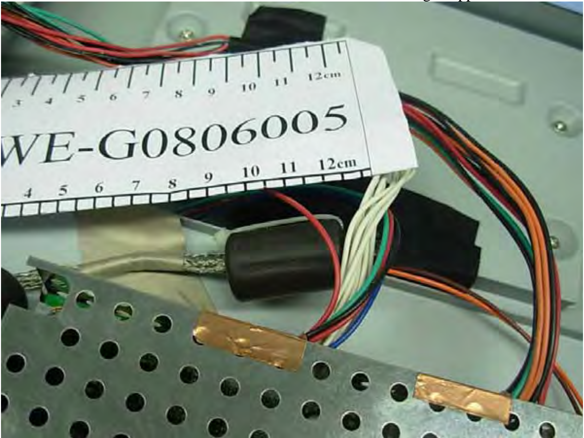
Figure 32 Conducting Copper Foil & Ferrite Core
