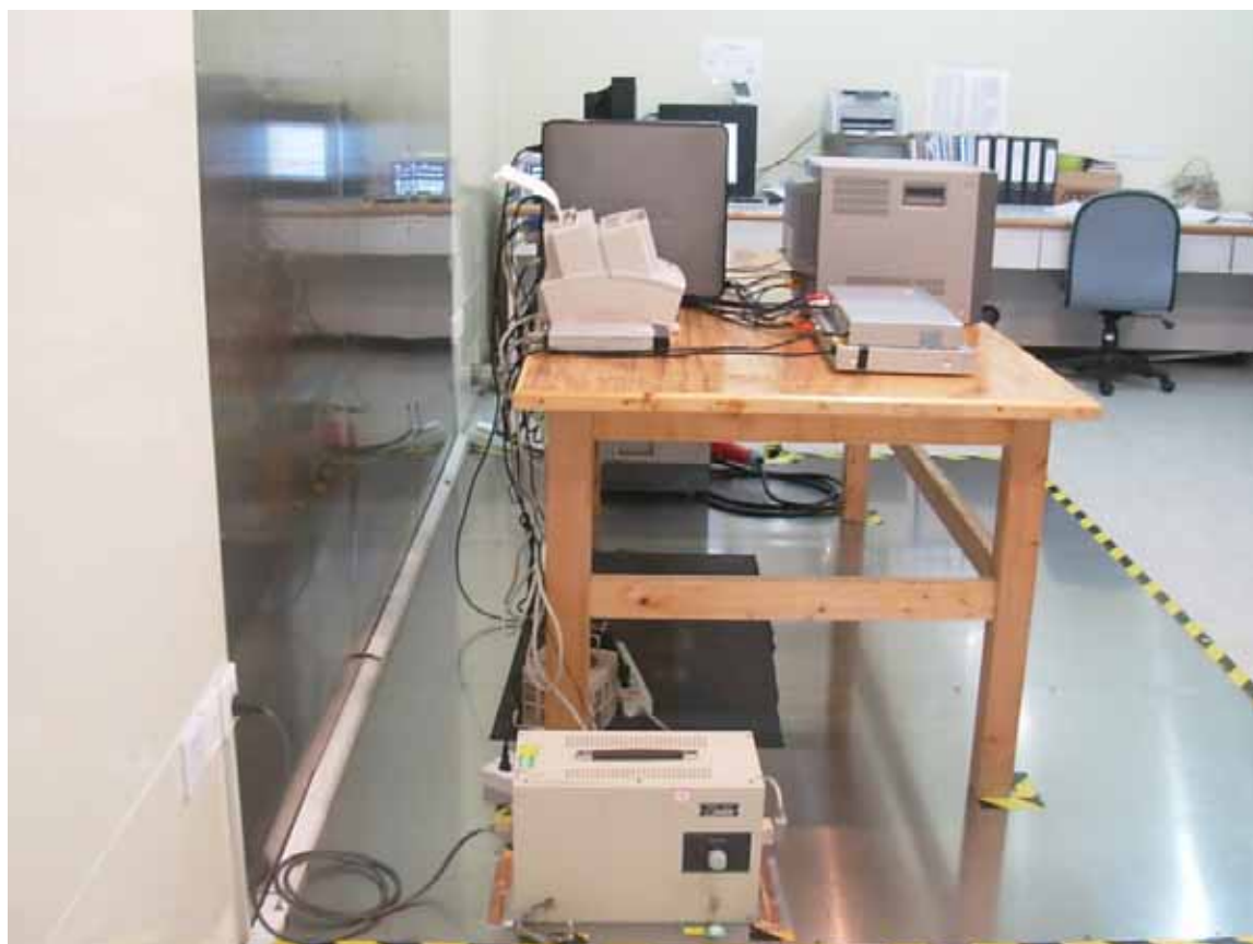
Side View of Conducted Emission Measurement (H Pattern)
