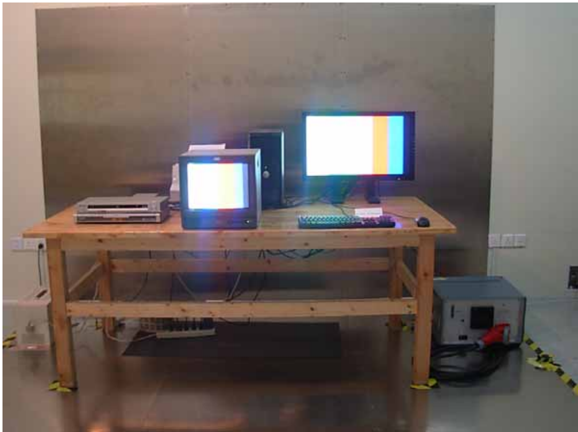
Front View of Conducted Emission Measurement (Colorbar)
