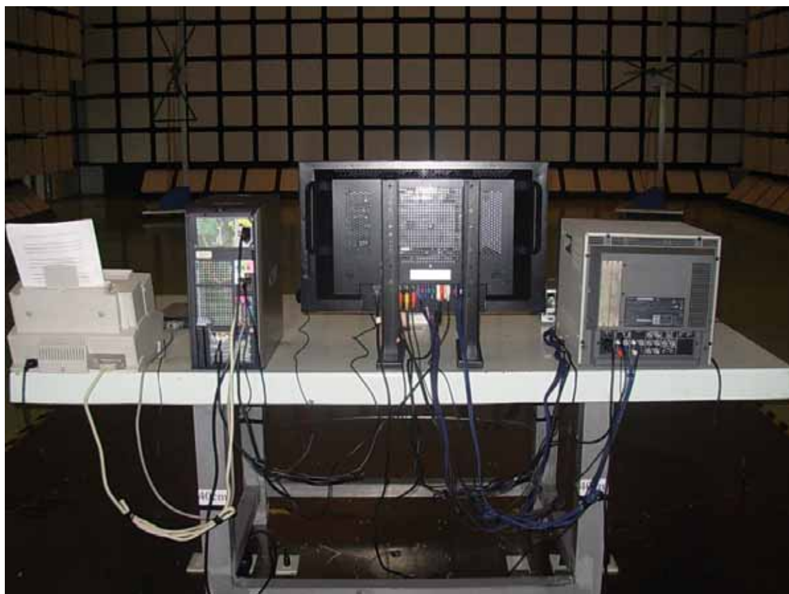
Back View of Radiated Emission Measurement (Colorbar)
