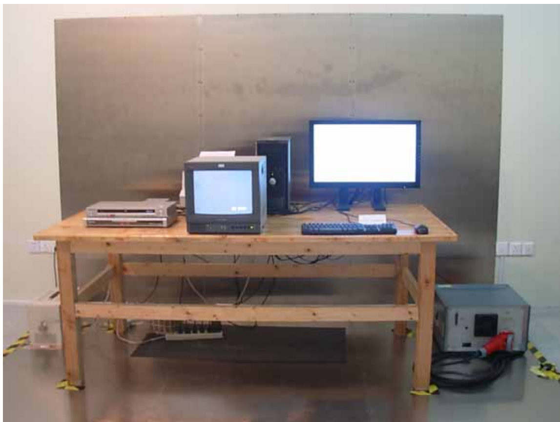
Front View of Conducted Emission Measurement (H Pattern)
