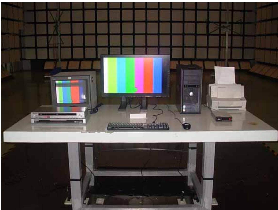
Front View of Radiated Emission Measurement (Colorbar)
