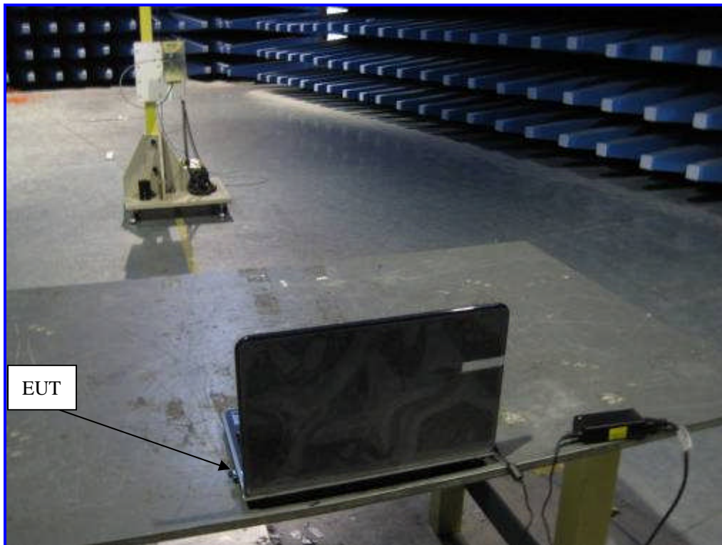
Radiated Emission Setup Rear View Above 1GHz
