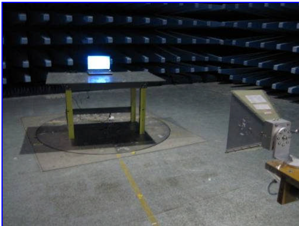
Radiated Emission Setup Front View Above 1GHz
