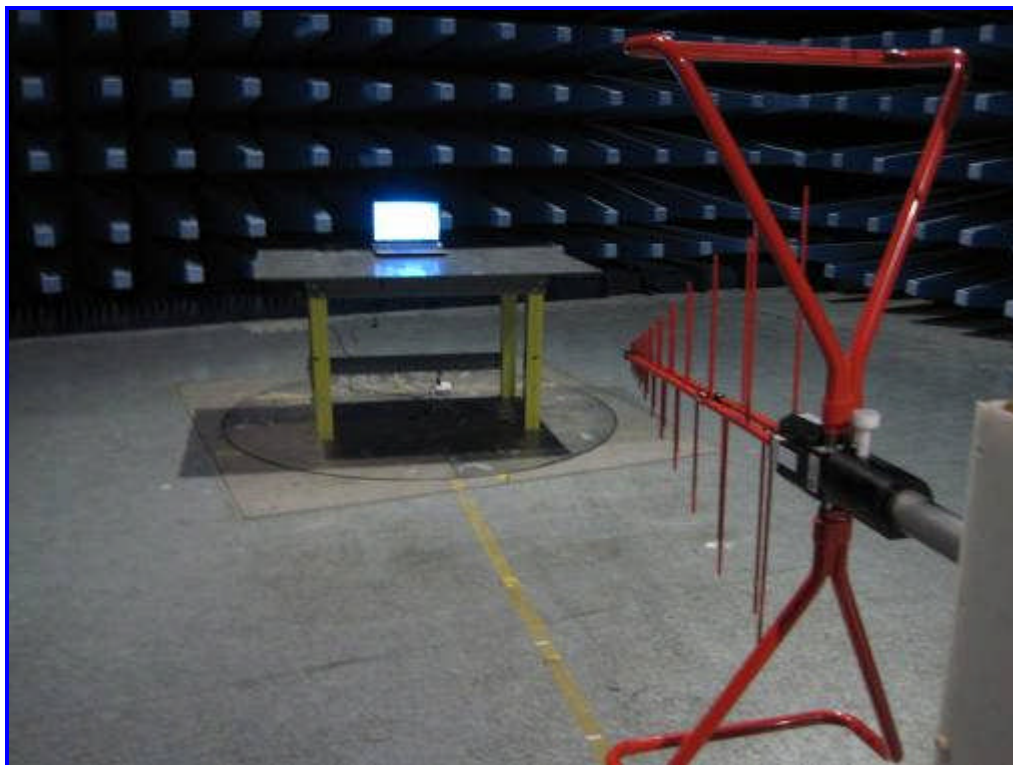
Radiated Emission Setup Front View below 1GHz
