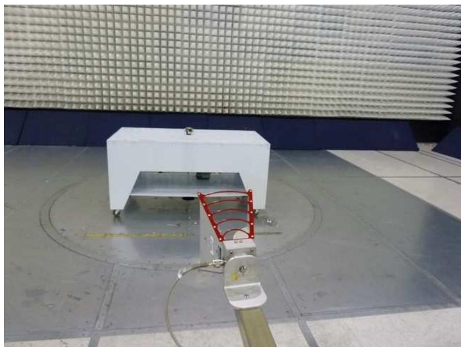
Radiated Emissions (Receiver spurious and Digital Parts)
