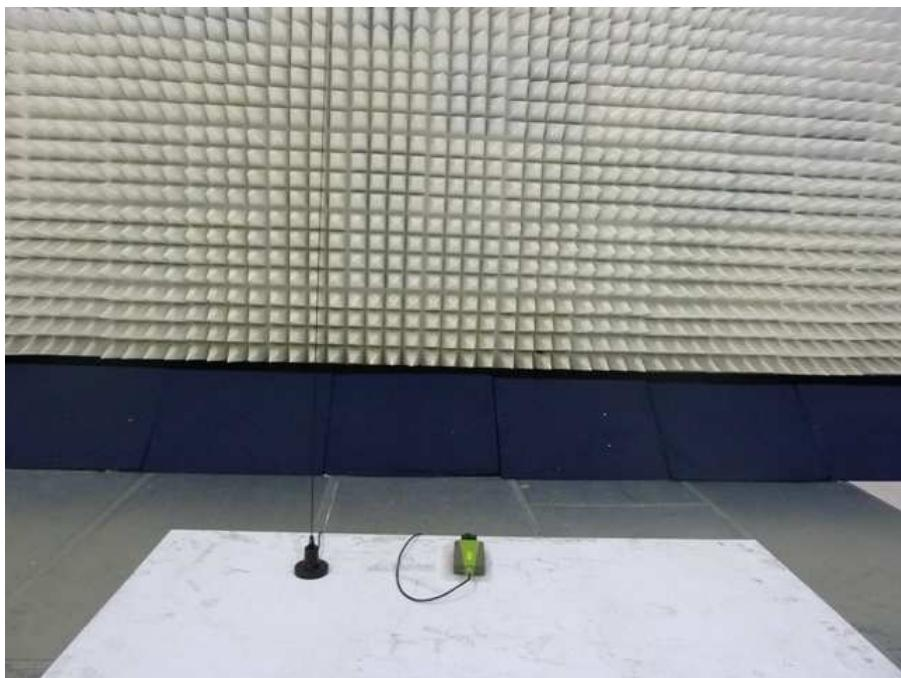
Radiated Emissions (Receiver spurious and Digital Parts)
