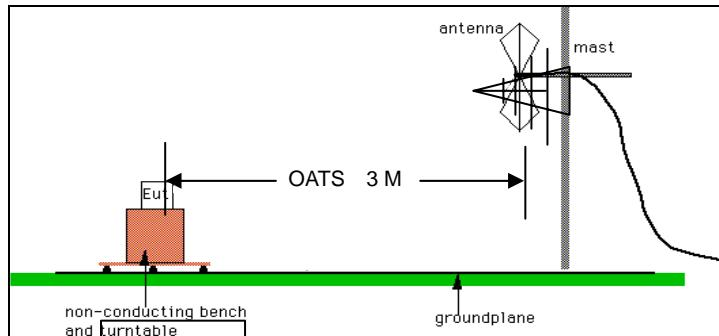
\* The radiated emission tests were performed in the 3 meters OATS(Open Area Test Site), using the Setup accordance with the ANSI C63.4-2003. The specification used was the FCC §15.231, §15.209 and §15.109
