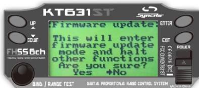
Prior activating this function, connect the USB cable between the back interface of the transmitter and a PC computer. A confirmation will be asked since all functions will be halted. Turn off any receiver before entering this mode. To exit this mode, simply turn off then back on the transmitter.
