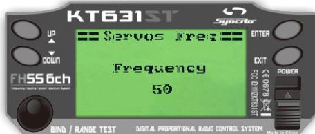
This function is used to set servo's frequency
