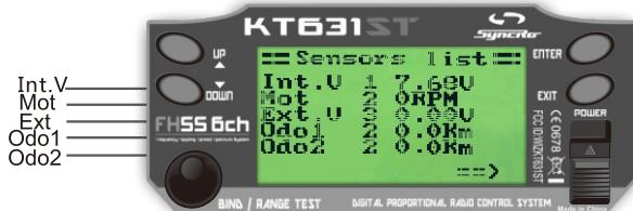
It shows all sensors' type, code and value, it can connect 15 sensors at most.
