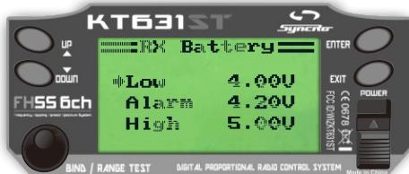
**Low voltage:** set the minimum voltage value. The battery is empty when the actual battery voltage value is lower than this value.
