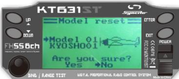
This function will reset the currently selected model to its default. The other models will not be affected. This can be useful when a setup is going nowhere and needs a fresh start. Since this function is destructive, a confirmation will be asked.
