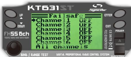
This function is used for setting the data of failsafe. Once the signal of receiver is lost, the one or more servos will back to pre-set position. "turn off" means the relevant servos will keep the last position when the signal is lost. Setting methods:
