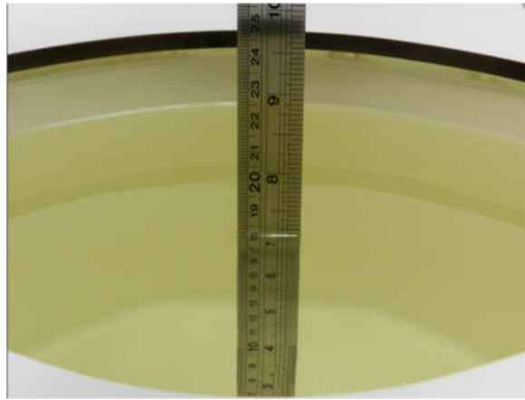
Fig 10.1 Photo of Liquid Height for Body SAR
