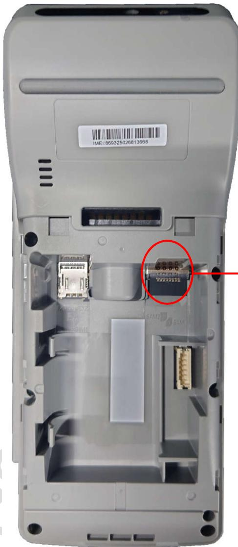
Step 1: Remove battery cover and battery
