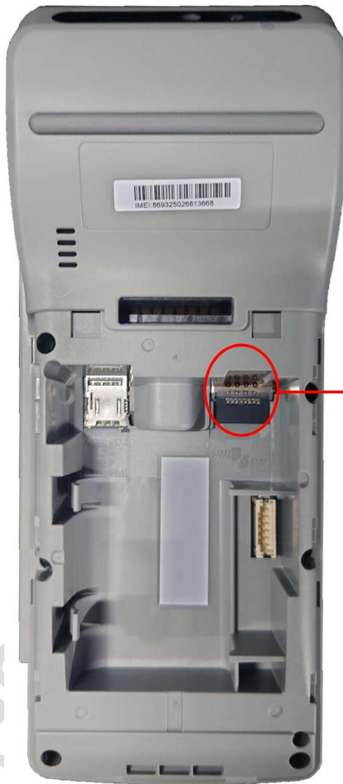
Step 1: Remove battery cover and battery
