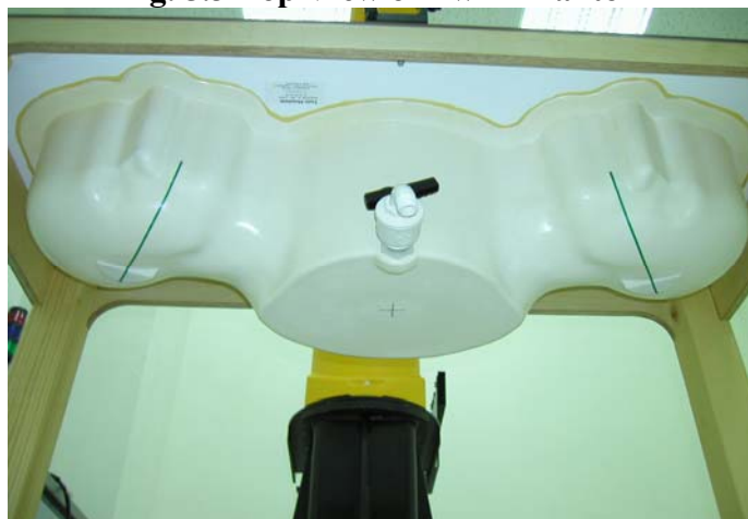
Fig. 5.4 Bottom View of Twin Phantom
