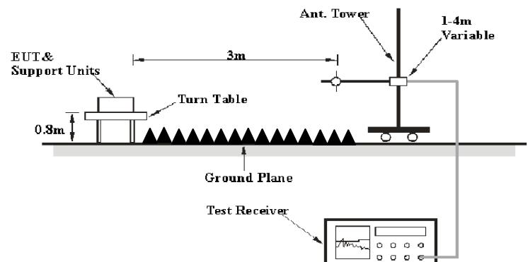
The radiated emission tests were performed in the 3 meters, using the setup accordance with the ANSI C63.4-2009. The specification used was the FCC 15.209, and FCC 15.407 limits.
