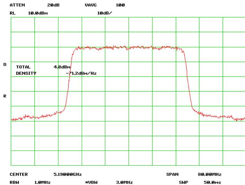
**Output Power-5190 MHz, Chain 1**
