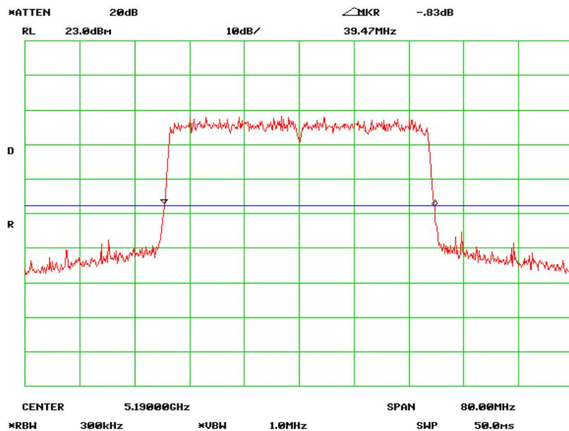
**26 dB Bandwidth-5190 MHz, Chain 1**
