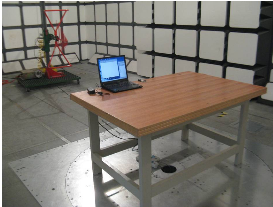
Below 1 GHz: Radiated Emissions - Rear View
