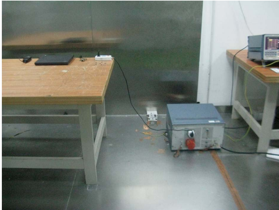
AC Line Conducted Emissions- Side View
