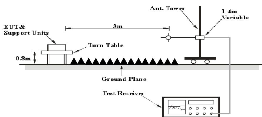
The radiated emission tests were performed in the 3 meters test site, using the setup accordance with the ANSI C63.4-2009. The specification used was the FCC 15.209, and FCC 15.407 limits.
