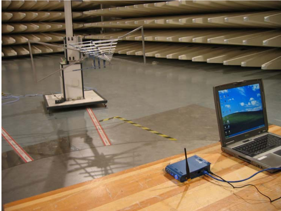
Photograph of Enclosure Radiated Emissions Test Setup
