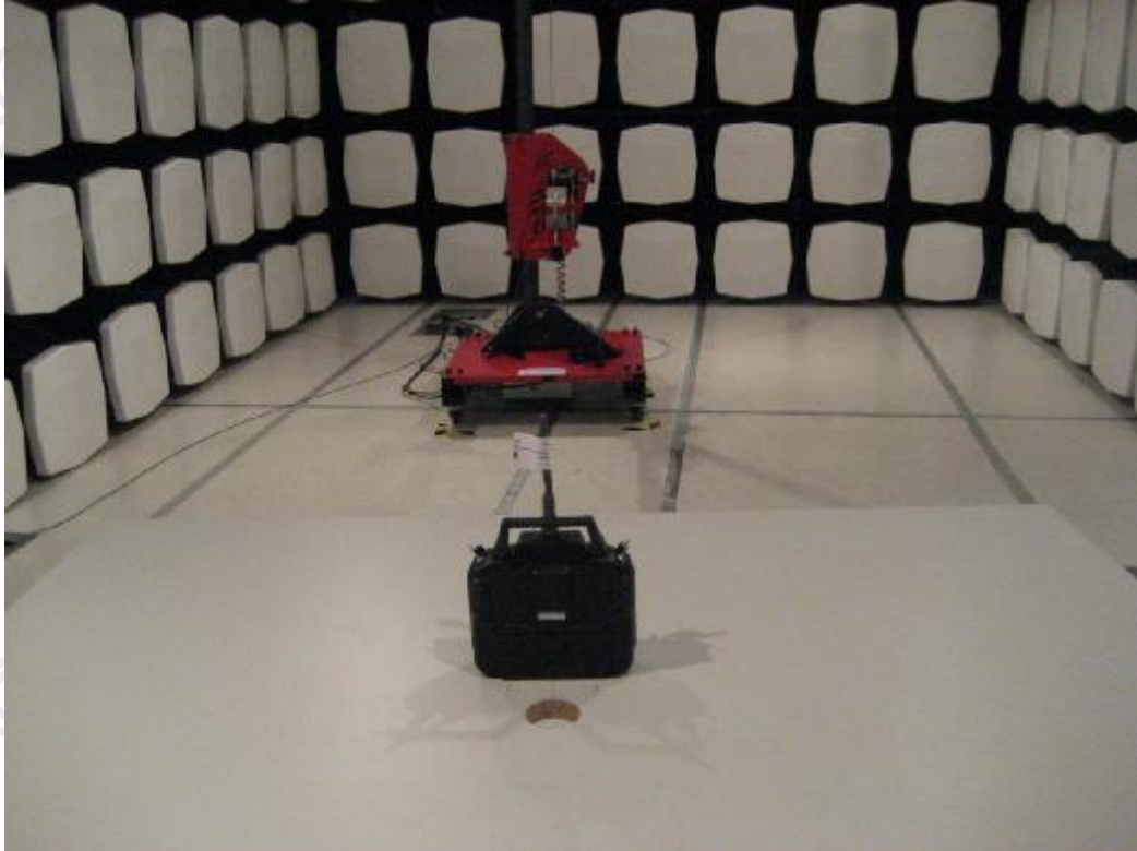
Measurement of Radiated Emission Test Set Up
