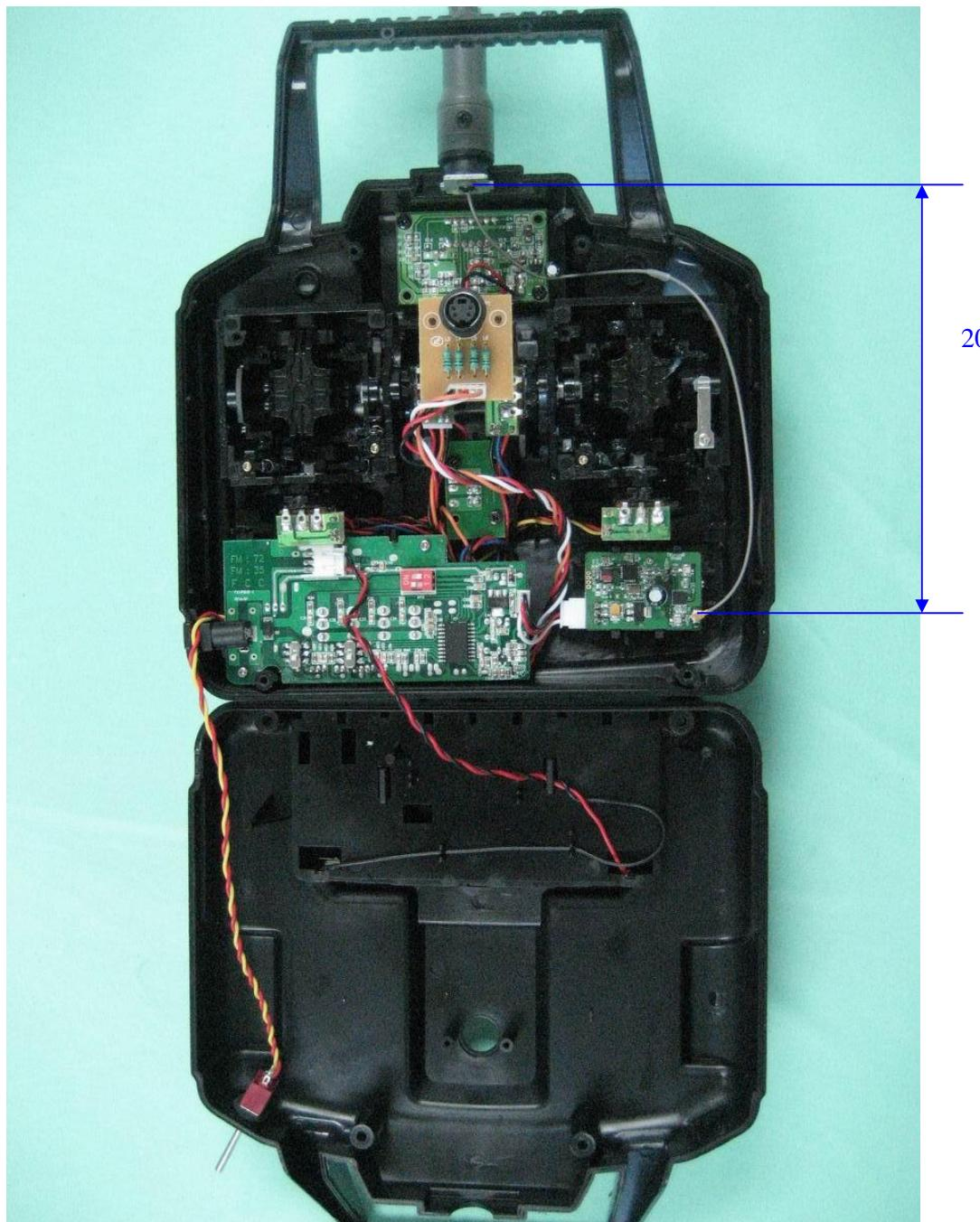
External antenna 14.5cm + Internal antenna 20.5cm = Total length is 35cm
