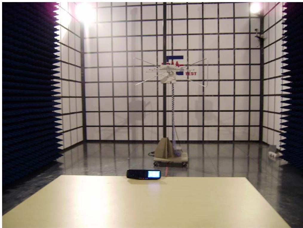
Radiation Emission Test Setup (Above 1GHz)
