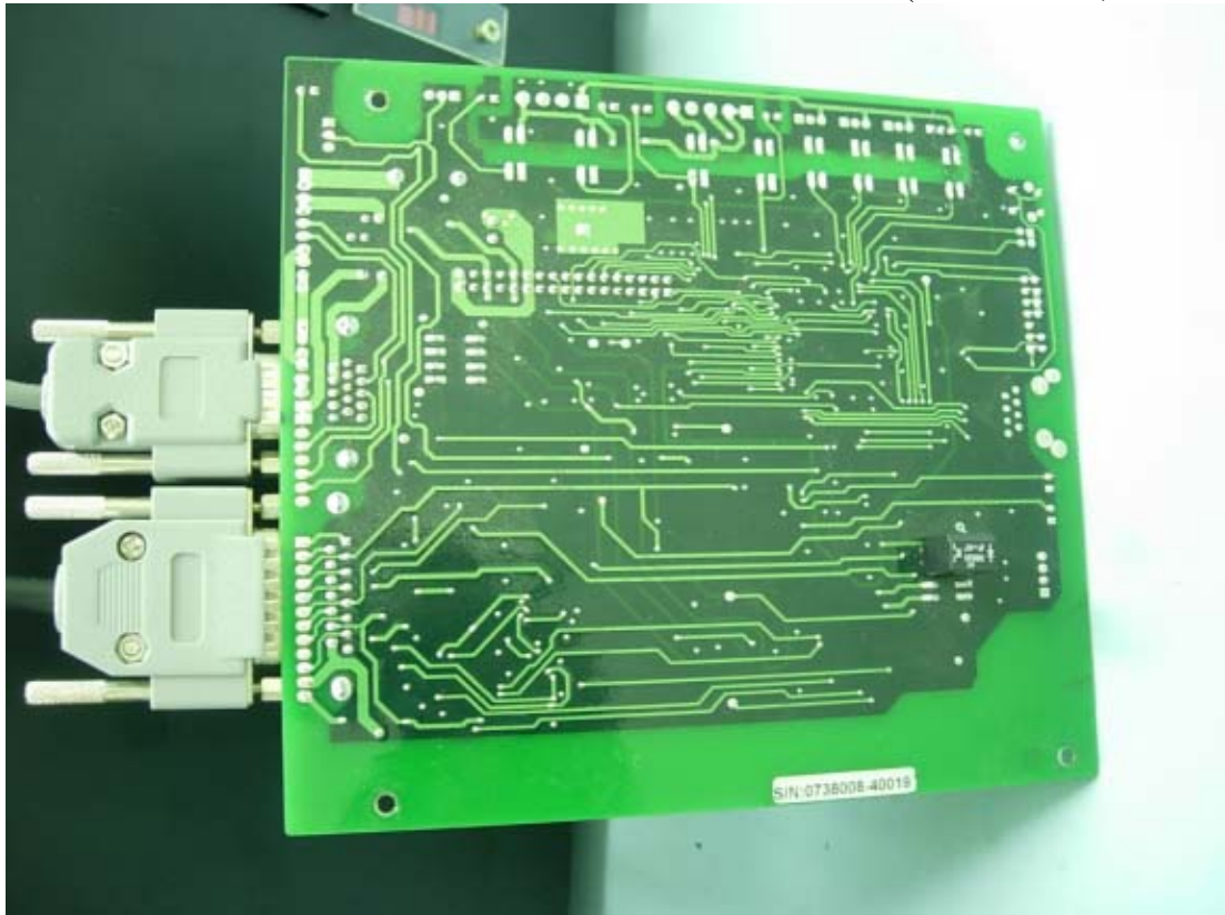
Figure 11 Internal View (Main Board, Back View)
