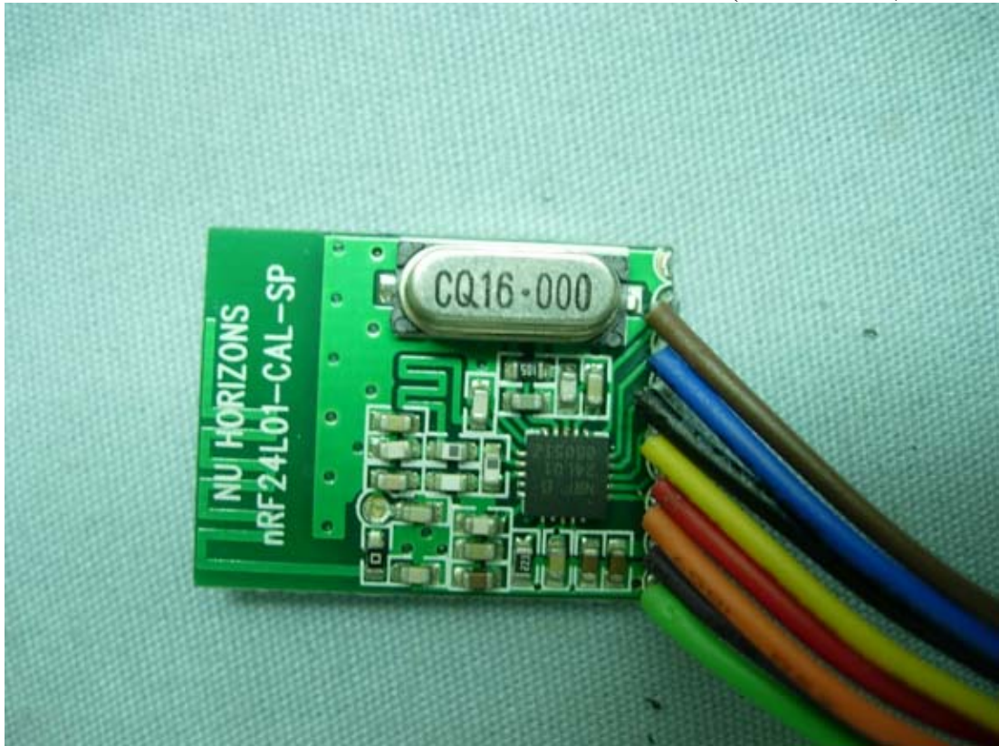
Figure 7 Internal View (RF Modular, Front View)
