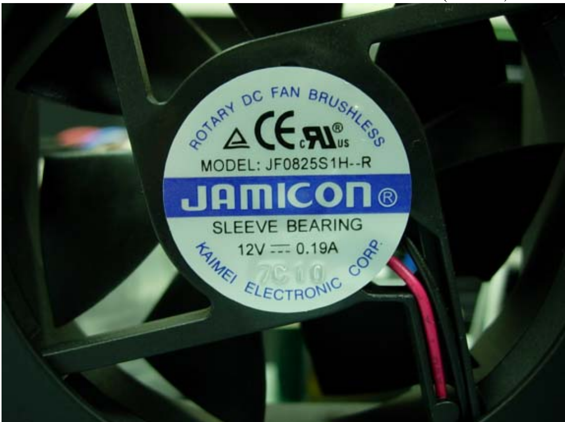
Figure 10 Internal View (DC Fan, Label View)
