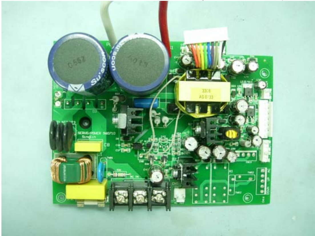
Figure 13 Internal View (Servo/Power Board, Front View)
