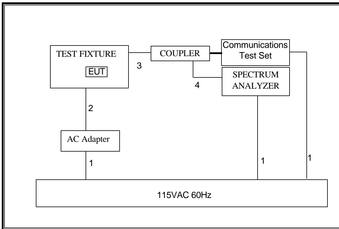
**SETUP DIAGRAM FOR RADIATED TESTS**
