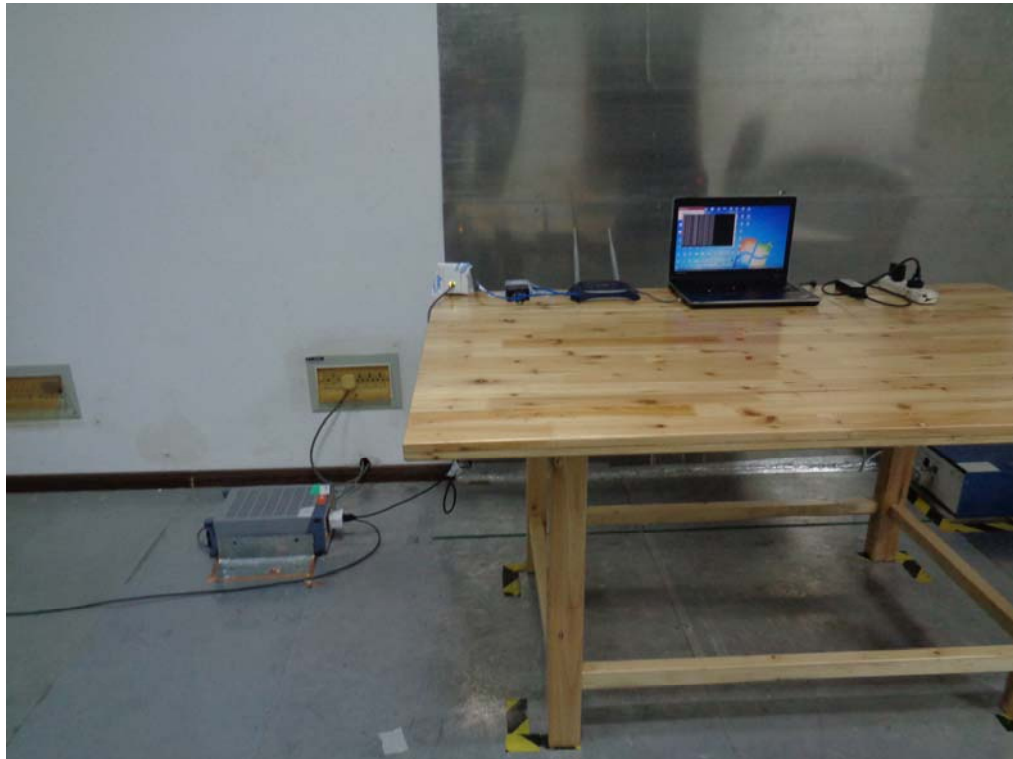
Conducted Emissions Setup Front View
