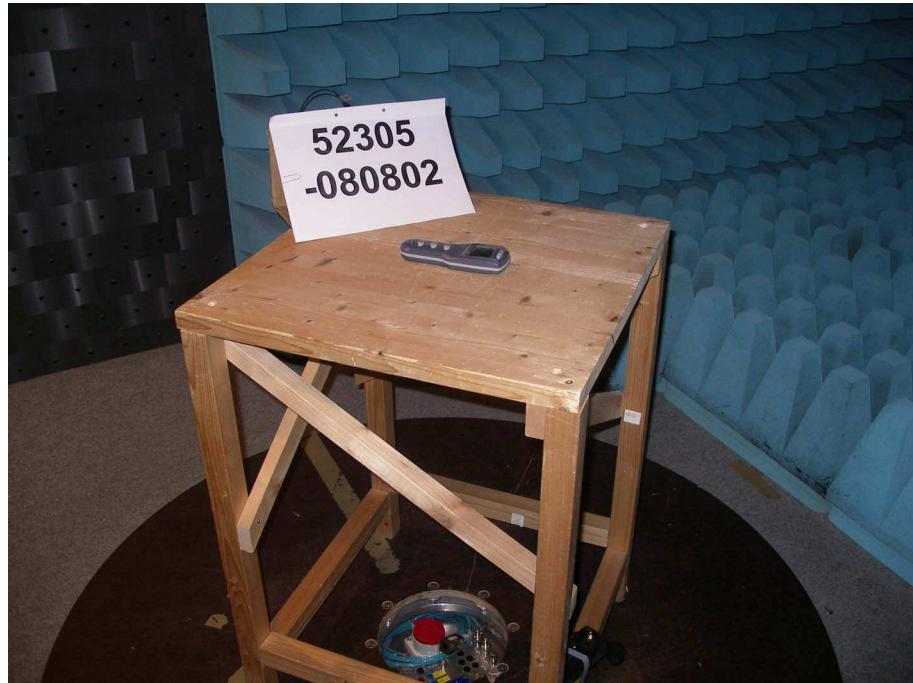
**Test setup for radiated emission measurement
