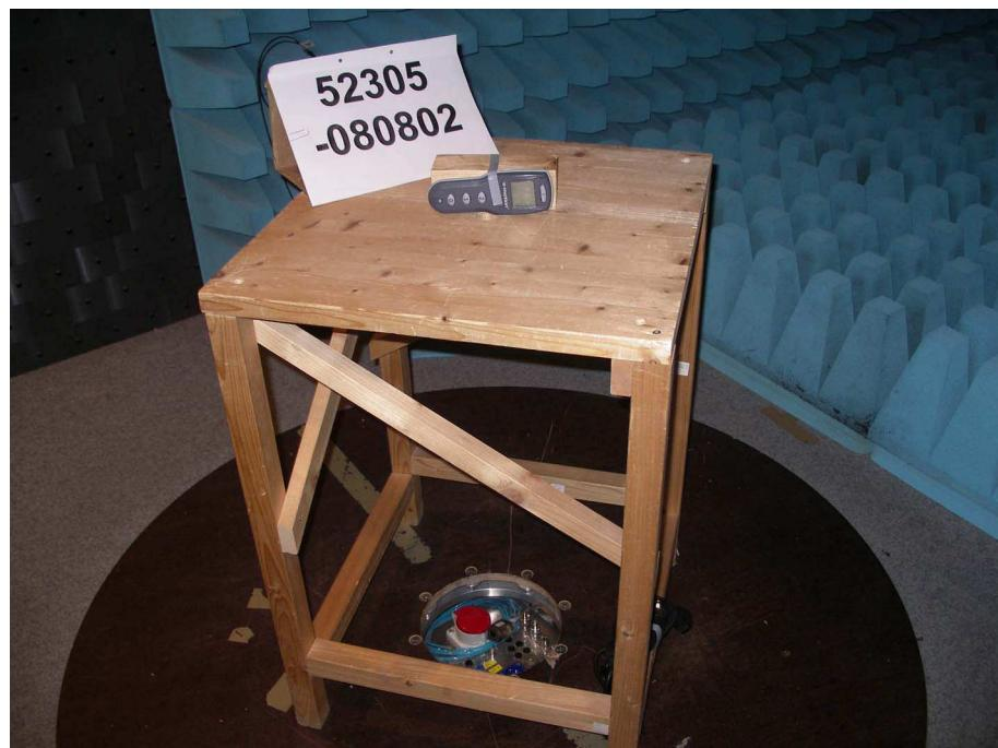
**Test setup for radiated emission measurement
