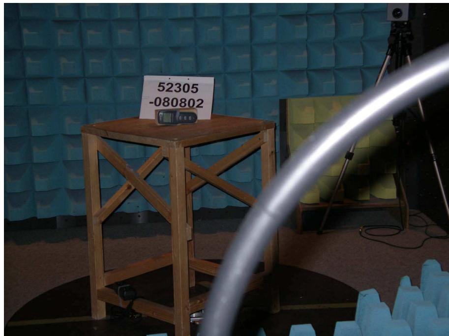
**Test setup for radiated emission measurement
