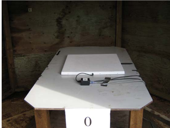
Emissions Test Setup of EUT Side View
