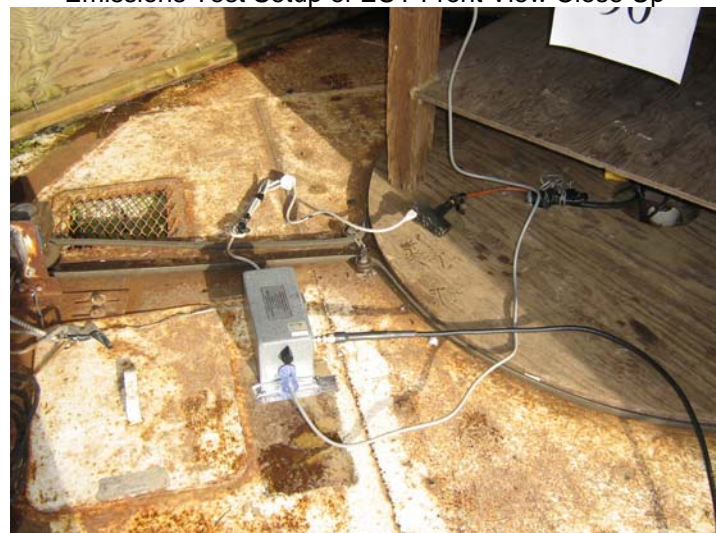
Emissions Test Setup of LISN used for Testing
