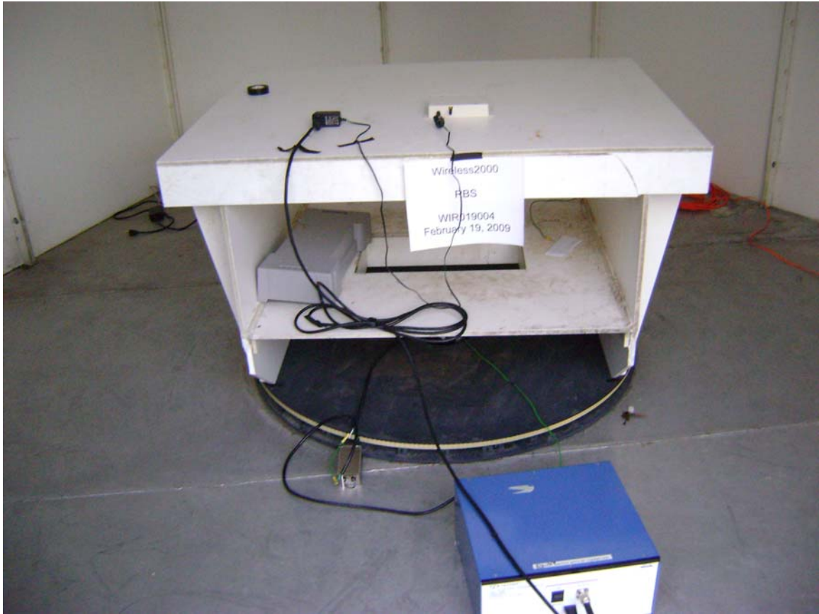
AC Mains Conducted Emissions Testing
