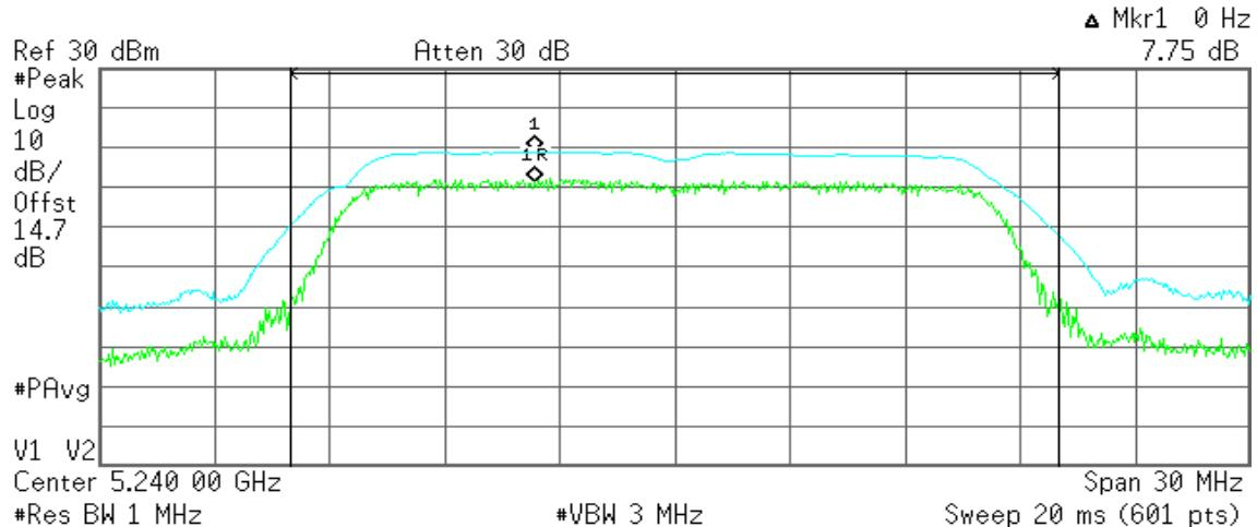
**IEEE 802.11n HT 20 MHz mode / 5180 ~ 5240MHz / Chain 0****CH Low****Agilent**
