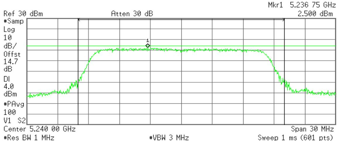
**Channel Power****12.22 dBm /20.0000 MHz****Power Spectral Density****-60.79 dBm/Hz****IEEE 802.11n HT 20 MHz mode / 5180 ~ 5240MHz / Chain 0****CH Low****Agilent**
