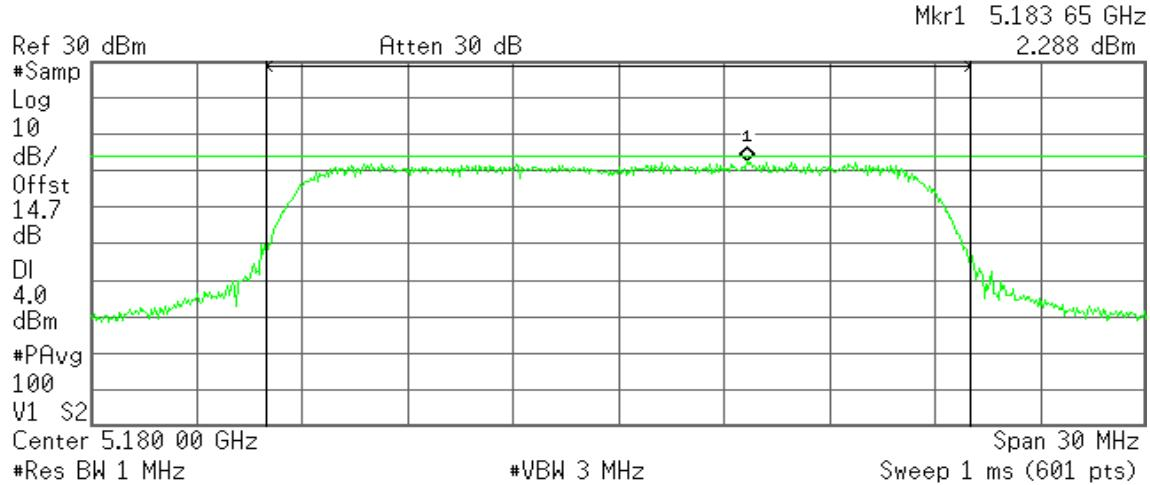
**Channel Power****12.33 dBm /20.0000 MHz****Power Spectral Density****-60.68 dBm/Hz**
