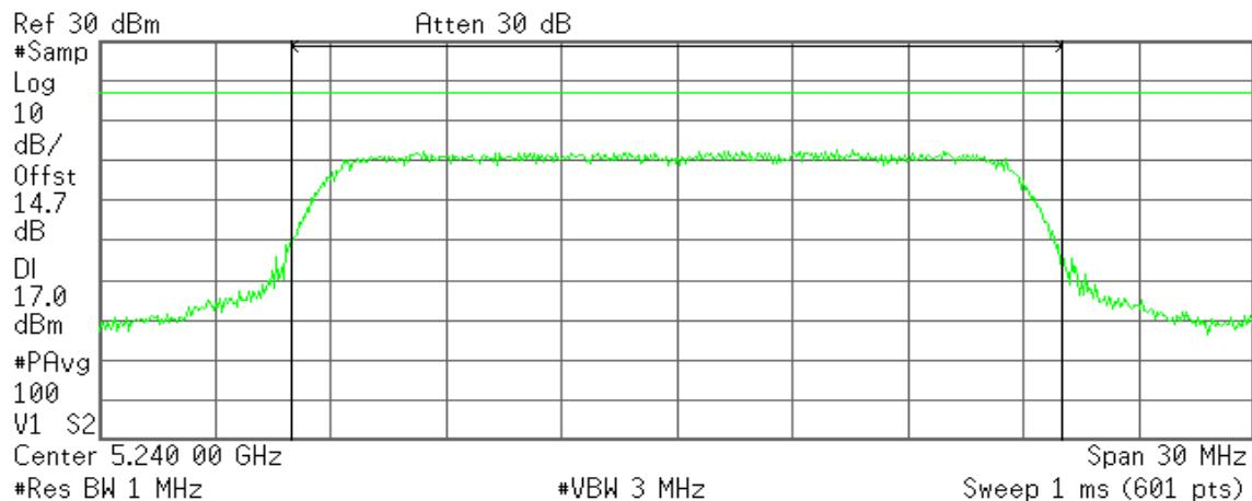
**Channel Power****13.34 dBm /20.0000 MHz****Power Spectral Density****-59.67 dBm/Hz**
