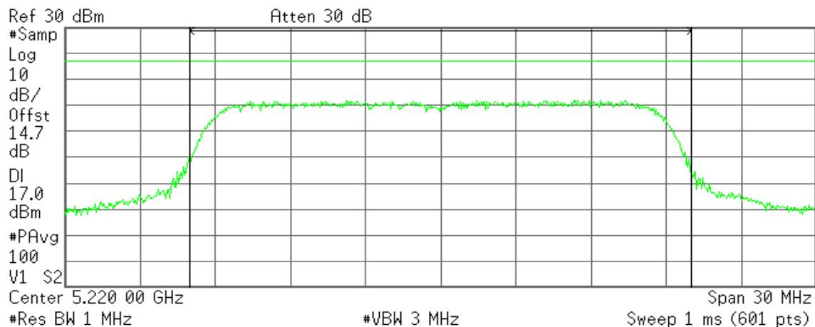
**Channel Power****12.46 dBm /20.0000 MHz****Power Spectral Density****-60.55 dBm/Hz****CH High****Agilent****R T**
