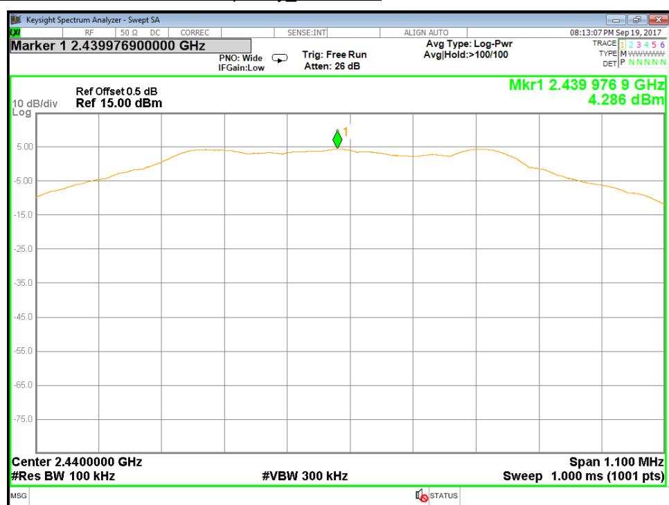
Test mode : Bluetooth LE / Middle Frequency Conducted Spurious Emission
