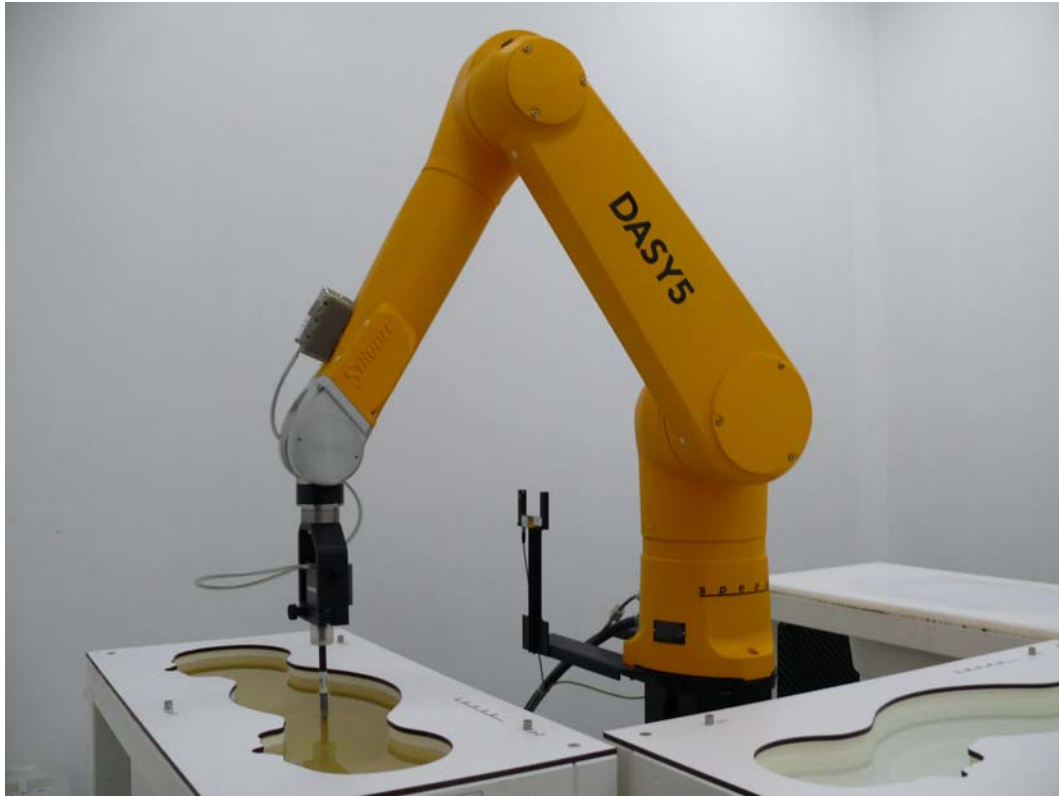
Picture 1: Specific Absorption Rate Test Layout
