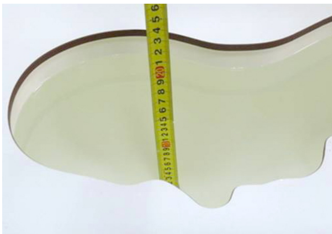
Picture 5: liquid depth in the head Phantom (1900 MHz, 15.2cm depth)
