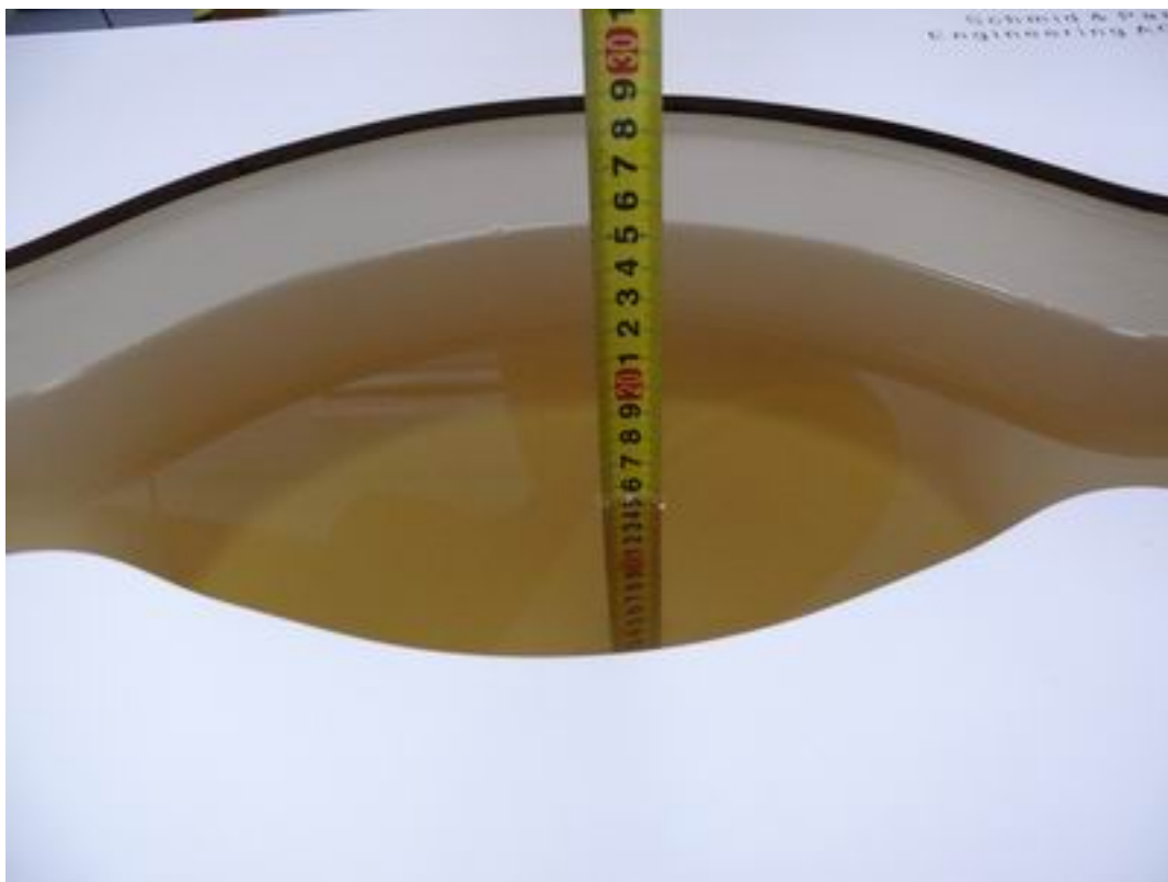
Picture 2: Liquid depth in the flat Phantom (835MHz, 15.3cm depth)
