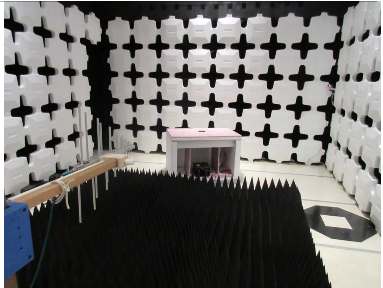
RADIATED EMISSIONS TEST SET UP PHOTO
