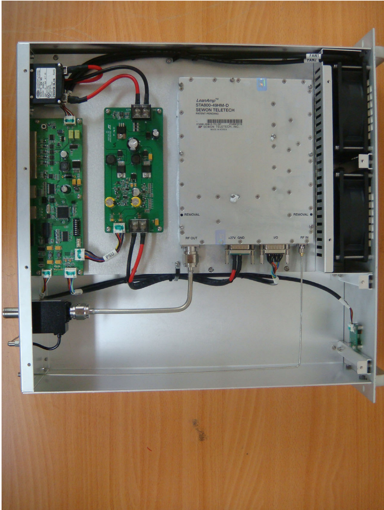
<Photograph 1: RU - Cover removed>
