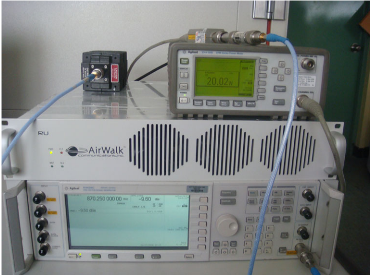
Figure 1: Photographs of the measurement of RF Power Output
